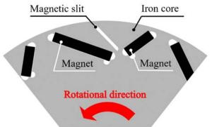
Asymmetric rotor structure of high-power-density motor
