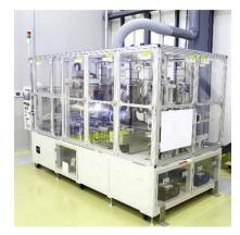
One-piece-flow automatic-sliding plating machine
