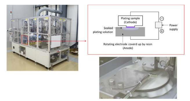
One-piece-flow automatic-sliding plating machine
