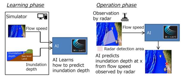
Learning and operation phases of radar-based AI for tsunami inundation depth prediction
