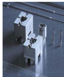
High-precision mold and the parts that compose it
