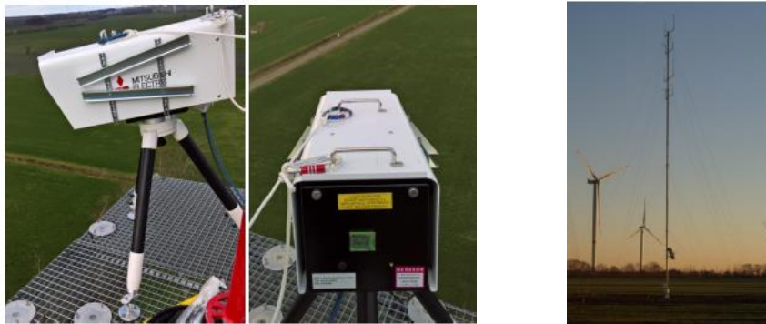
Photos of DIABREZZA lidar (left), and DNV GL test site in Janneby Germany (right)
