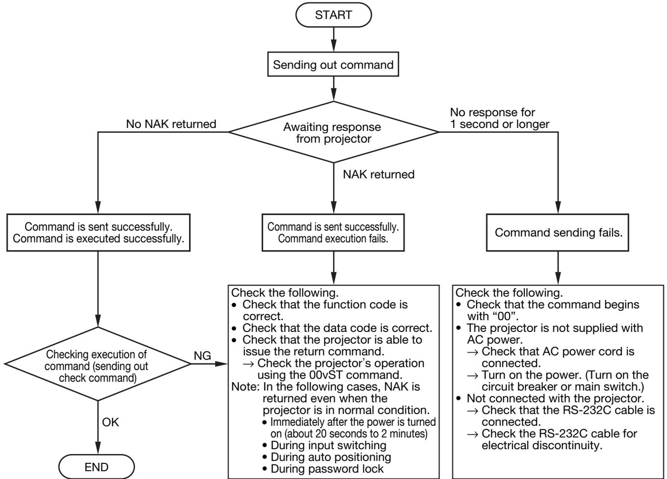
**[Method of checking state of projector]**
