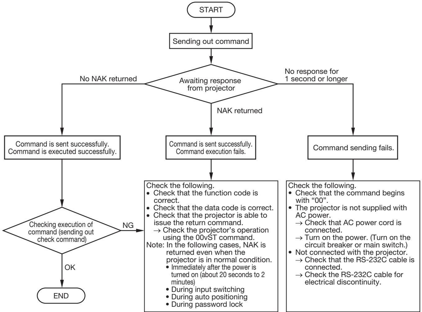
**[Method of checking state of projector]**
