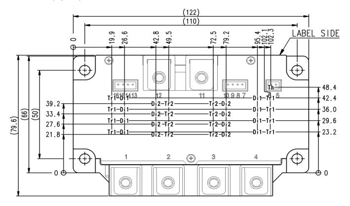
Tr1,Tr2: SiC-MOSFET, Di1,Di2: SiC-SBD, Th: NTC thermistor
