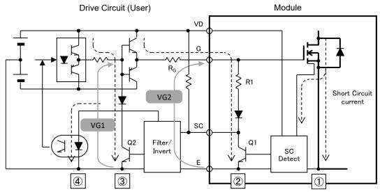
Example of application (Short circuit detection & protection)
