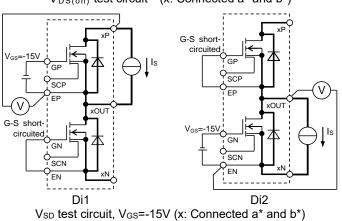
V<sub>SD</sub> test circuit, V<sub>GS</sub>=15V (x: Connected a\* and b\*)
