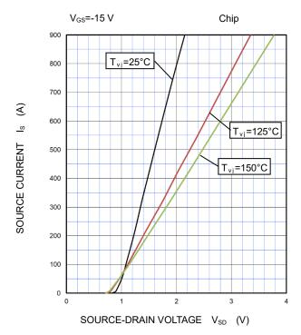
SOURCE-DRAIN ON STATE VOLTAGE CHARACTERISTICS (TYPICAL)
