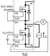
$V_{DS(on)}$  test circuit (x: Connected a\* and b\*)
