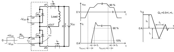
Switching characteristics test circuit and waveforms(x: connected a\* and b\*)
