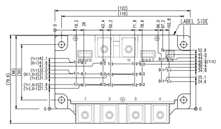
Tr1,Tr2: SiC-MOSFET, Di1,Di2: SiC-SBD, Th: NTC thermistor
