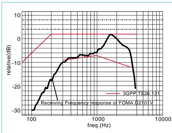
Fig. 4 Receiving frequency response for the TS26.131 and the FOMA D2101V
