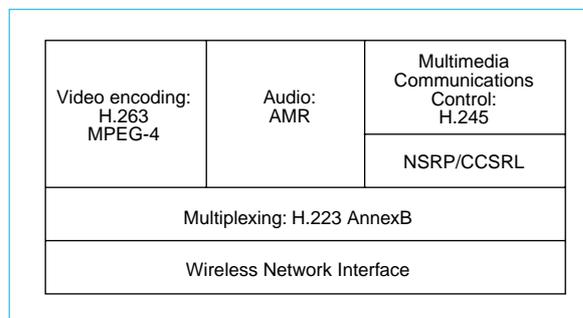
Fig. 1 Protocol stack for 3G-324M multimedia system video encoding: H.263 MPEG-4
