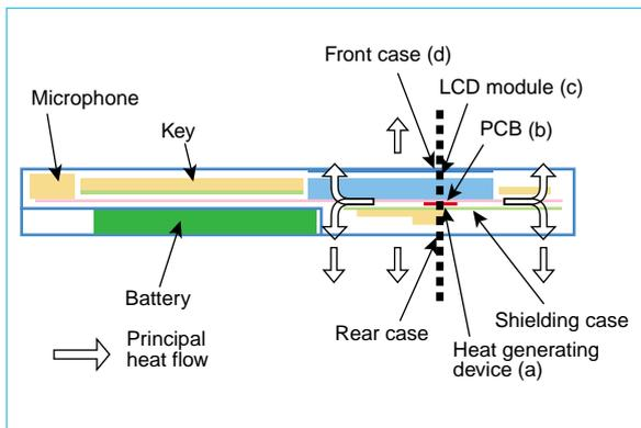
Fig. 4 Schematic cross-sectional diagram of a mobile phone
