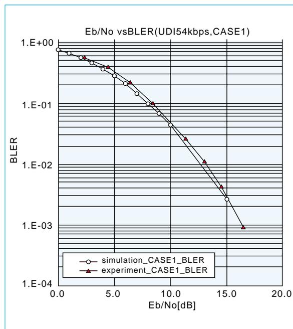
Fig. 3 Block error rate (BLER) of the prototype unit
