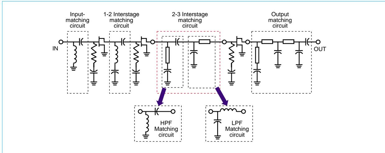
Fig. 4 Schematic diagram of the three-stage HPA module using the high pass filter/low pass filter combined interstage matching circuit developed in this development project
