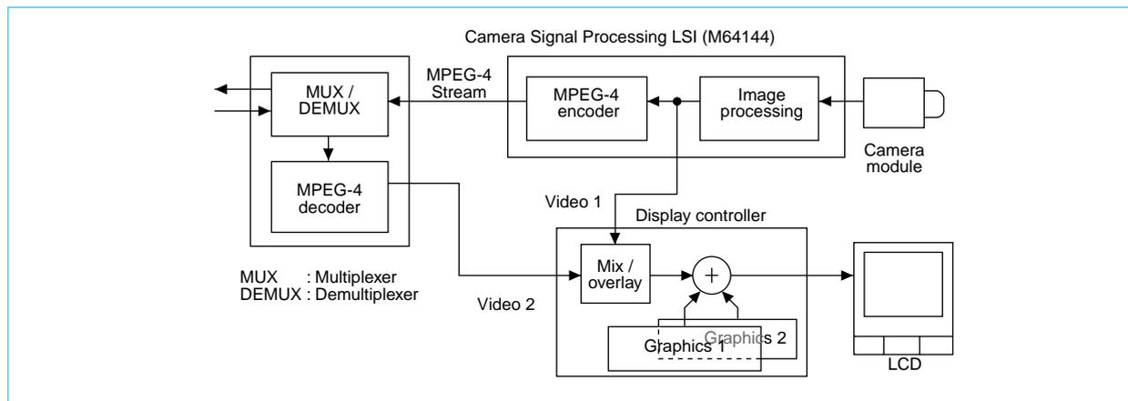
Fig. 1 Total block diagram for video-system processing
