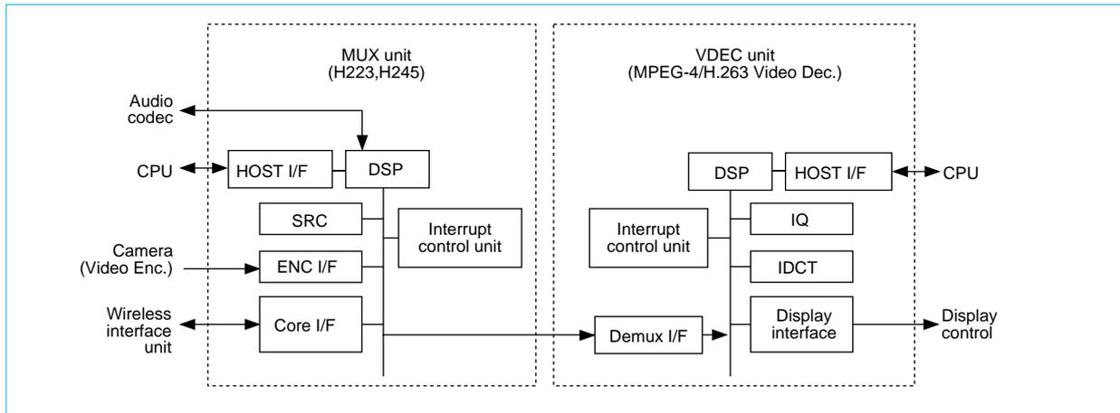
Fig. 4 Block diagram of the 3G-324M IC module
