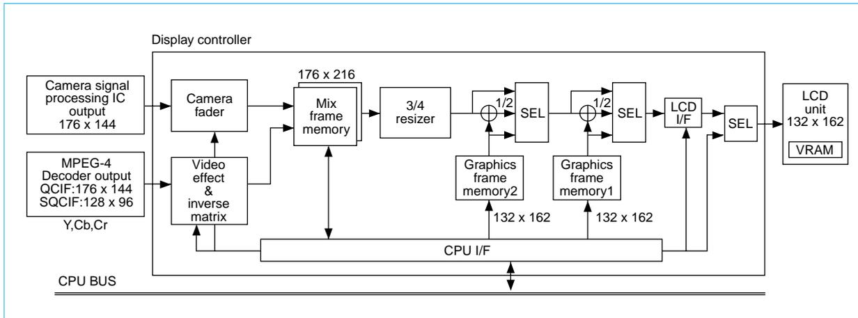
Fig. 3 Clock diagram of display controller
