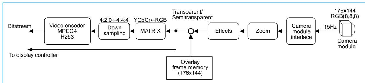
Fig. 2 Block diagram of camera signal processor LSI
