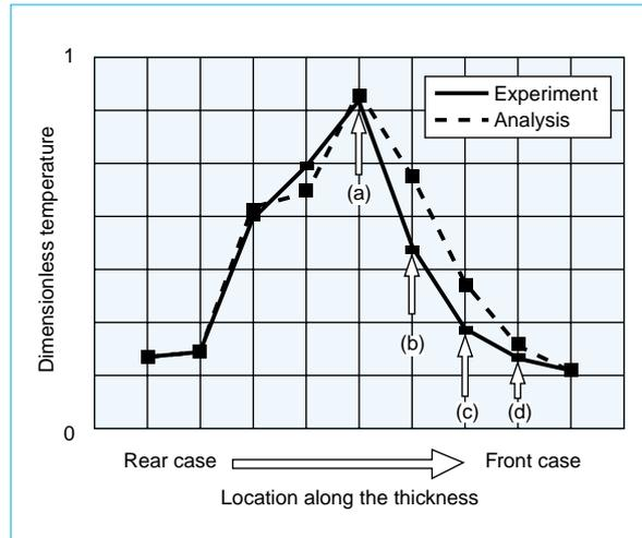
Fig. 5 Temperature distribution along the thickness of a mobile phone
