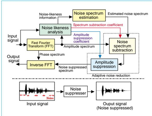
Fig. 2 Block diagram of the noise suppresser
