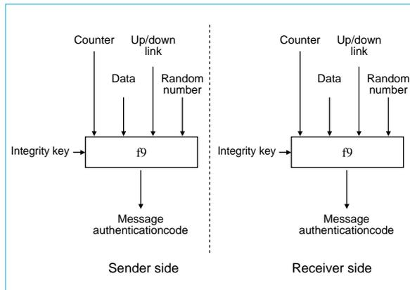
Fig. 3 Function  $f_9$  to insure data integrity
