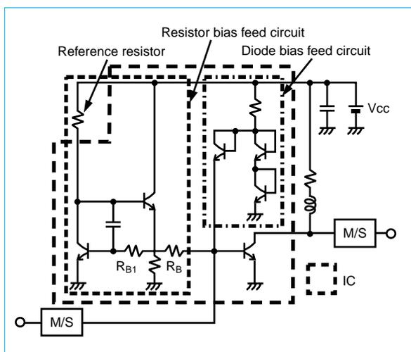
Fig. 2 Schematic diagram of dual-bias feed LNA
