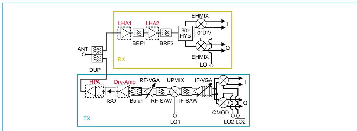
Fig. 1 Block diagram of RF section
