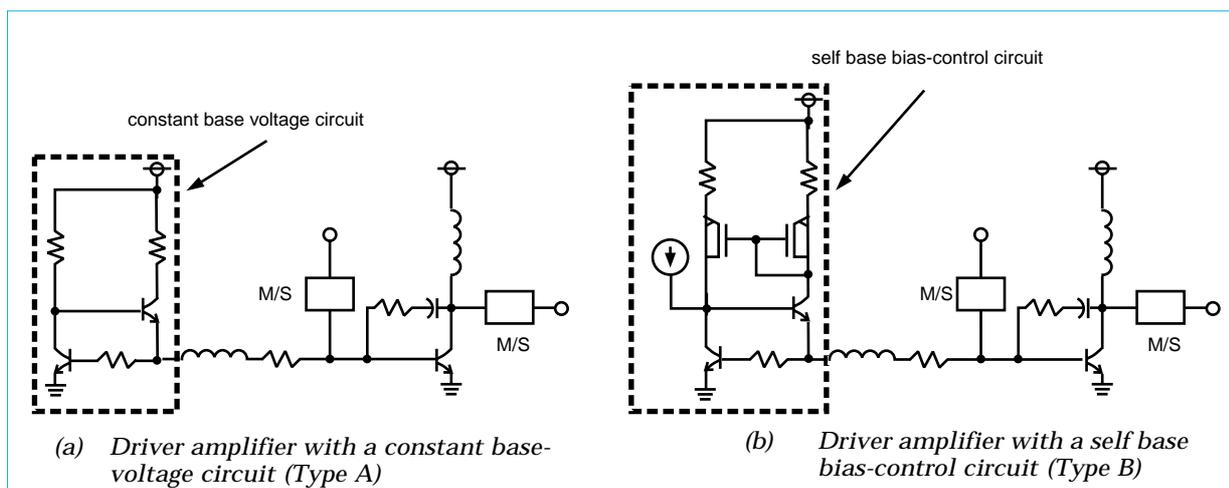
Fig. 3 Schematic diagram of driver amplifier
