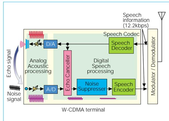
Fig.1 Block diagram of the W-CDMA mobile phone
