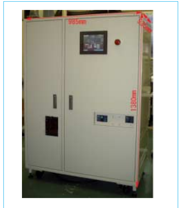
Fig. 4 PFC abatement equipment for RIE tools.
