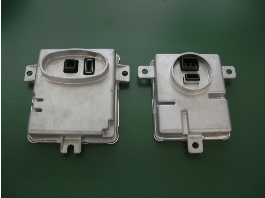
Fig. 4 Ballast for a conventional bulb (left) and ballast for the mercury-free bulb (right)
