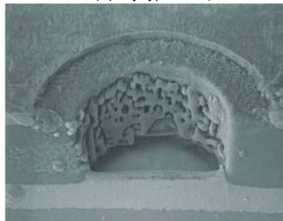
φ100-µm large window processing (Glass-epoxy resin)
