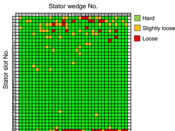
Fig. 4 Typical robotic inspection result (wedge tightness inspection)
