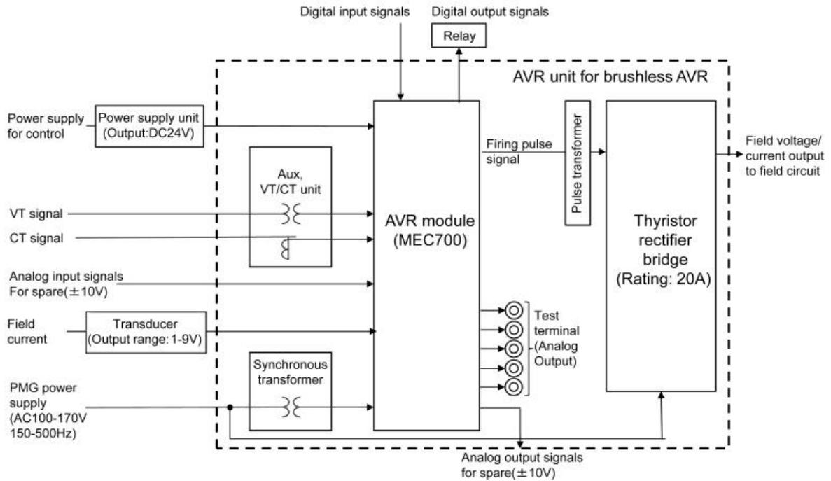
Fig. 11 System configuration of MEC700 digital AVR unit
