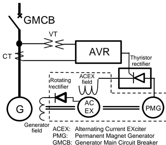
Fig. 1 Brushless excitation system configuration
