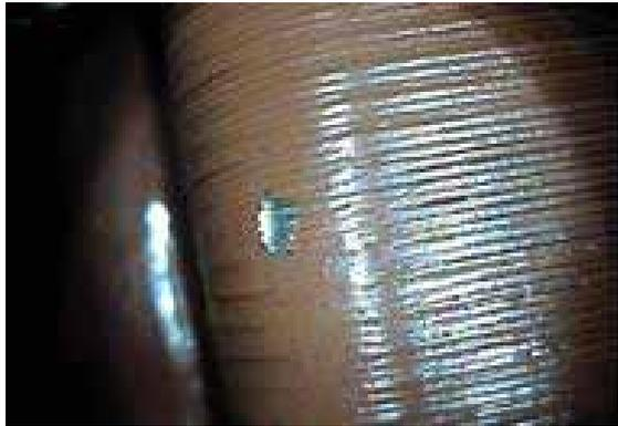
Fig. 3 Typical robotic inspection result (using a remote camera)–damage on a stator core
