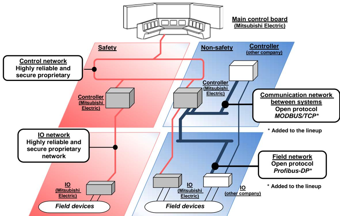
Fig. 4 Typical network configuration
