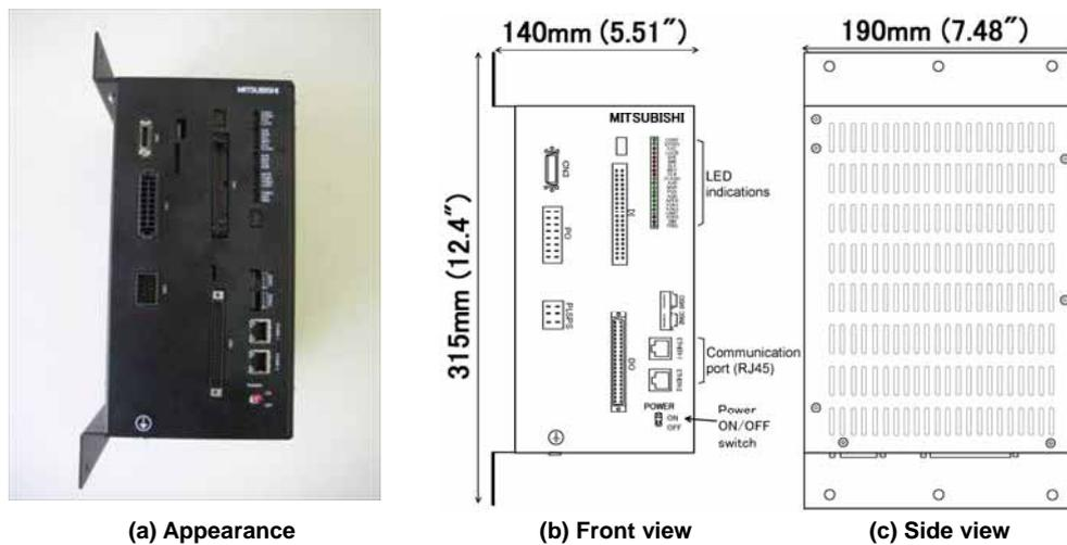
Fig. 9 Appearance of the latest digital AVR (MEC700) module
