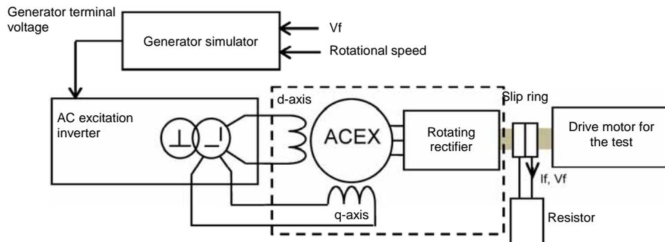
Fig. 12 Circuit for the assembly test
