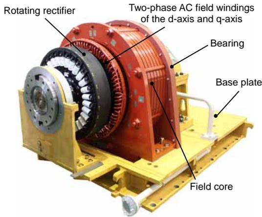
Fig. 8 Prototype of the AC field winding brushless exciter (after installation of the rotor)
