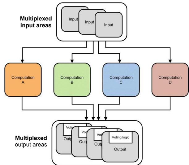
Fig. 2 Typical SIL3 system configuration
