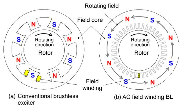
Fig. 7 Magnetic field structures of AC exciters
