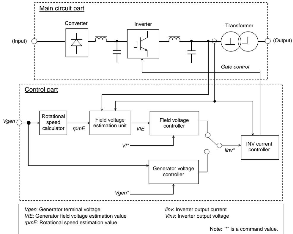
Fig. 11 Circuit block diagram of the inside of the AC excitation inverter
