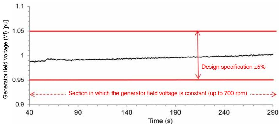
Fig. 13 Test results of the generator field winding voltage estimation control
