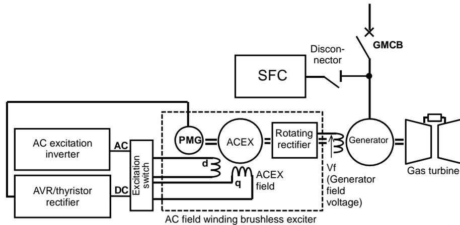
Fig. 6 Circuit of the SFC starting and AC field winding brushless excitation system
