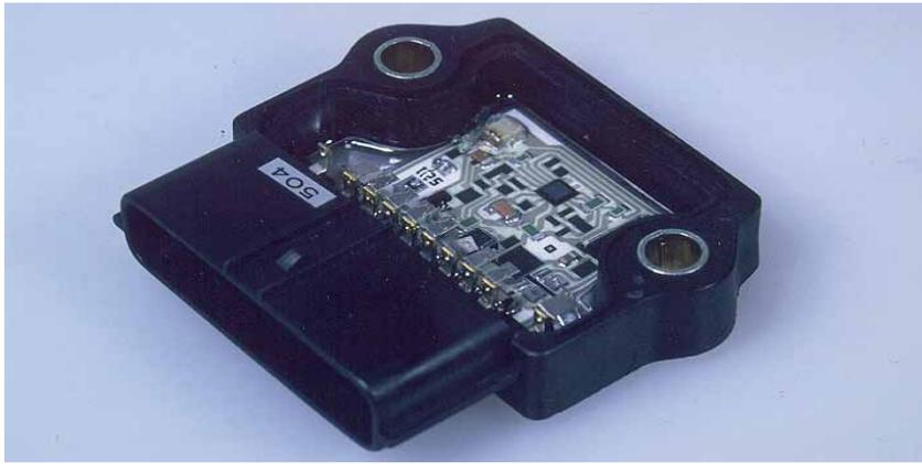
The ionic current detection module.
