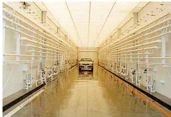
Fig. 3 Natural environment simulation facility.
