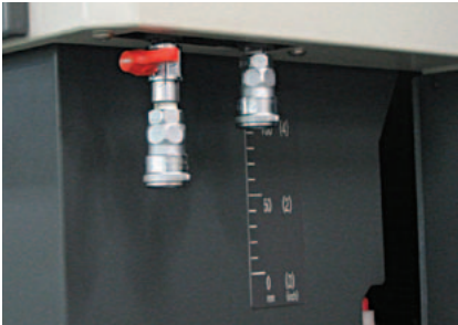
Sprays dielectric fluid between workpiece and electrode during pitch machining.
