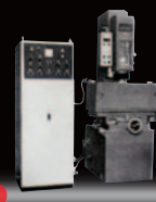
Transistor pulse power supply DM250+DE30T 1967
