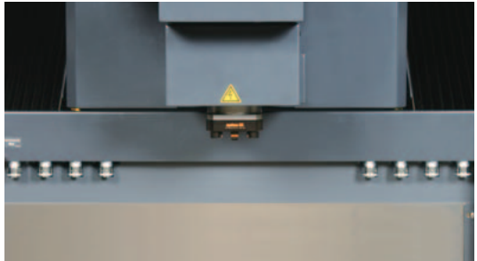
Fluid treatment for multiple set-up machining etc (set either emission or suction for coupler and sequentially execute with NC program). (photo shows EA12V ADVANCE specifications)
