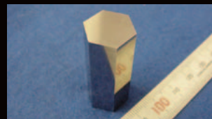
Glossy mirror finish machining Electrode: Copper Workpiece: Steel (STAVAX) Surface roughness: Rz:0.4μm/Ra:0.06μm
