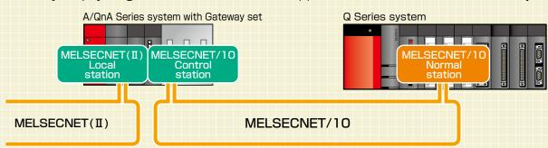
[Example] Step-by-step system replacement to have a system entirely made up with the Q Series
