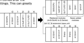
Replace the modules, which cannot be installed with the Q Series modules.
