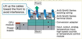
• If the cables still interfere, leave an empty slot between modules to secure wiring space.
