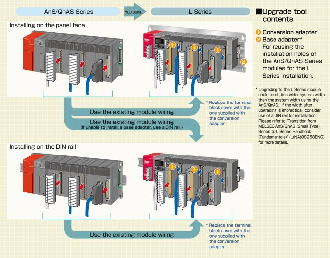
Note 1: Use of the L Series space module may restrict the system configuration. Please refer to "MELSEC-L CPU Module User's Manual (Hardware Design, Maintenance and Inspection)" (SH-080890ENG) for the detailed specifications, precautions and restrictions.
