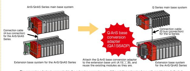
The conversion adapter is connected to the extension connector area of the existing extension base unit, requiring no dedicated extension space.
