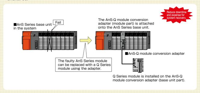
●Up to three AnS-Q module conversion adapters (module part) can be installed on one base unit.
