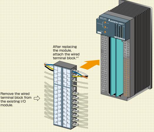
\*1: The communication cables and power cables need to be rewired.
