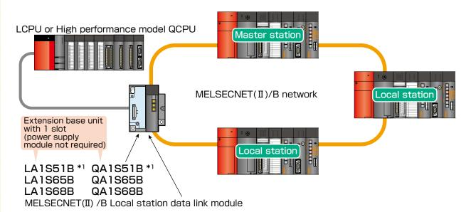
\*1: LA1S51B/QA1S51B are not equipped with the extension cable connector (OUT). No further extension can be made from the LA1S51B/QA1S51B. LA1S51B/QA1S51B cannot be used with LA1S6□B, QA6□B, and QA6ADP+A5□B/A6□B.
