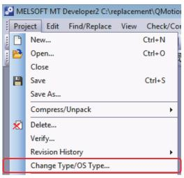
2) Select the replaced Motion CPU (the setting example below: Q173DSCPU) for "Type" and the new operating system software type for "OS Type". Click "OK".
