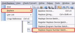
2) Select "Replacing with specified K/F/G program range" tab. Enter the device numbers in [Replace From:] [To:], and [Replace With:]. Click [Check >> Execute].
