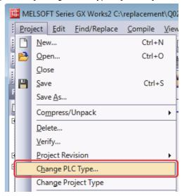
3) Select the replaced PLC CPU model for "PLC Type" (the setting example below: Q06UDV). Click "OK".
