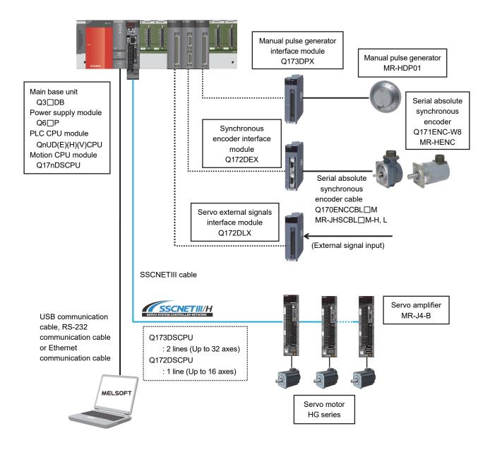
Note) There is a restriction on installation position of Motion modules (Q172DLX, Q172DEX, Q173DPX). Refer to 2.4.2 (3) for details.
