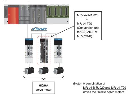
(2) When the HC/HA servo motor has malfunctioned Simultaneously replace the servo amplifier and the malfunctioned servo motor.
