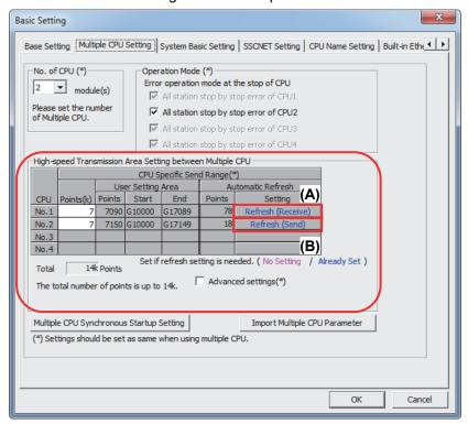
(b) Click (A) and (B) on the screen above, and check the detailed settings of the automatic refresh.
