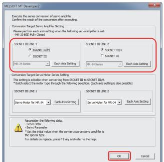
Execute the series conversion of the servo amplifier. Select the network to be used (SSCNET type) for the replaced servo amplifiers (for Q17nDSCPU), and click [OK].
