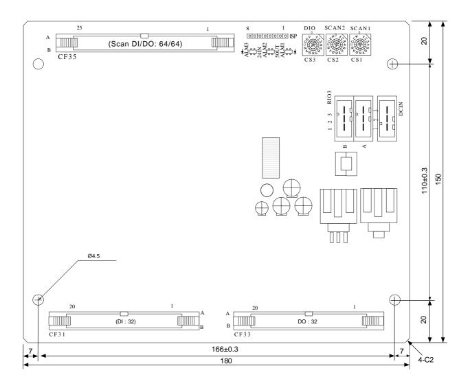
\* The PCB height (depth) will be approx. 40mm when the connector is inserted, so secure a space larger than that during installation.
