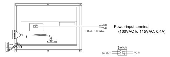
Use a double-OFF type that completely cuts off the circuit when turning the power ON and OFF.
