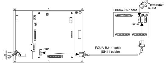
Refer to the explanation on each I/O item for details on setting the number of stations, etc. When connecting the remote I/O, always connect a terminator (R-TM) to the final station. Refer to the "PLC Interface Manual" for details on the interface assignments.
