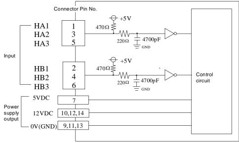
The power voltage supplied to the manual pulse generator can be changed between 5VDC and 12VDC by changing the cable wiring. Supply the power from pin 7 for the 5VDC power supply manual pulse generator, and from pins 10, 12 and 14 for the 12VDC power supply manual pulse generator. Use several power and 0V (GND) wire materials in the cable.
