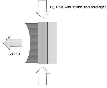
d) For the screw fixed type connector, loosen the two fixing screws, and pull the connector off.
