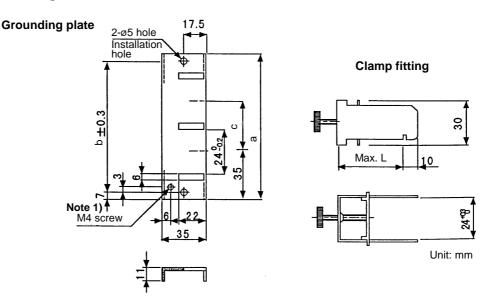
(Note 1) Screw hole for wiring to cabinet's grounding plate. (Note 2) The grounding plate thickness is 1.6mm.
