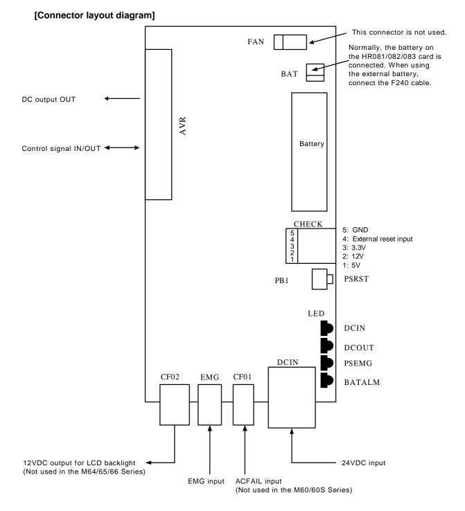
PSRST: System reset (do not press during normal system operation)
