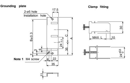
Note 1) Screw hole for wiring to cabinet's grounding plate
