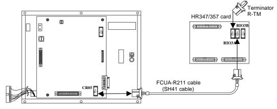
Refer to the explanation on each I/O item for details on setting the number of stations, etc. When connecting the remote I/O, always connect a terminator (R-TM) to the final station. Refer to the "PLC Interface Manual" for details on the interface assignments.
