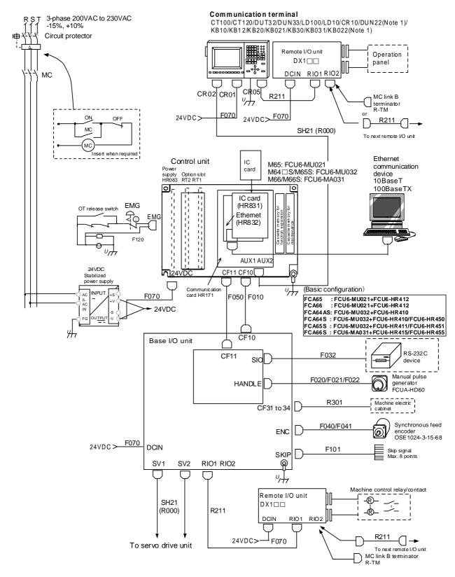
The R200 cable can also be used for the +24V power supply cable F070. The R000 cable can be used for the servo drive unit's communication cable and communication terminal's communication cable SH21.
