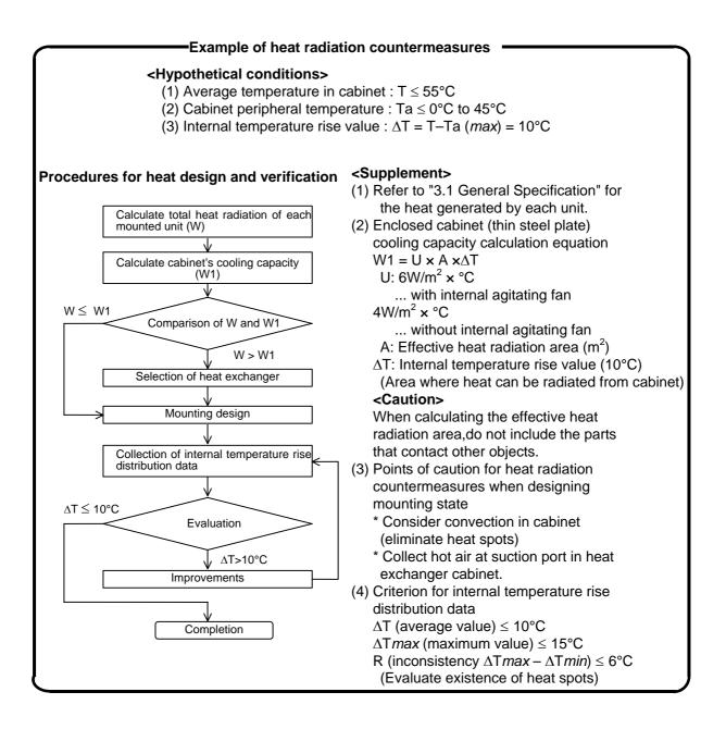
The following shows an example of heat radiation countermeasures for the operation box. Because heat will accumulate in the upper portions of the communication terminal, install an agitating fan as required.
