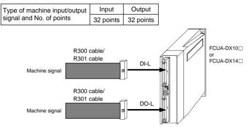
The remote I/O unit cable types include the R300 and R301 types. The R300 cable has one end cut off, and the R301 cable is used for connection to the IDEC IZUMI Corporation terminal block BX1F-T40A<sup>(Note 1)</sup>. The R300-3M and R301-3M cables are available. If a cable longer than 3m is required, use the CN300 and CS301 connector set.
