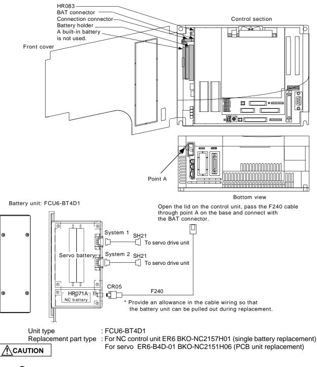
• If the battery voltage drop warning alarm occurs, the programs, tool data and parameters could be damaged. Thus, reload each data with the input/output device after replacing the battery.
