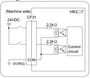
**Input conditions** Set so the input conditions are within the ranges shown in the following conditions.
