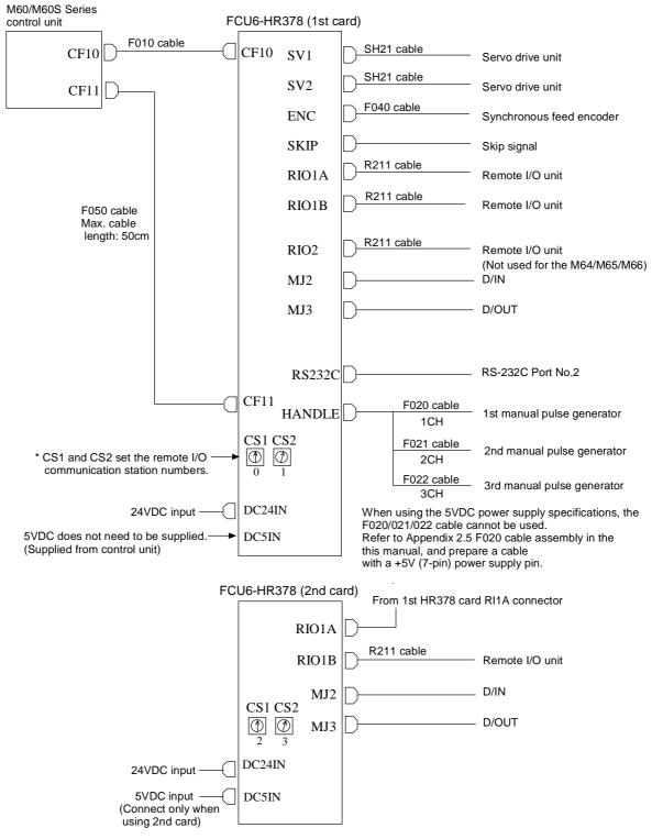
\* When using two FCU6-HR378 cards, the 5VDC for the second card must be supplied from an external source as it is not supplied from the control unit.
