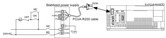
Turn the control unit power ON after turning or simultaneously with the turning ON of the peripheral units (servo drive unit, remote I/O, etc.).
