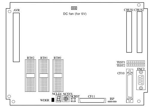
TEST 1 & 2 : Test pins for maintenance and serviceNCRST: NC reset (do not press during normal system operation)
