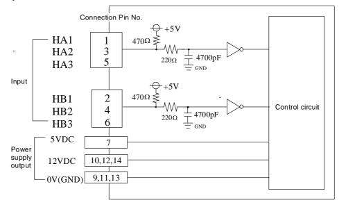
The power voltage supplied to the manual pulse generator can be changed between 5VDC and 12VDC by changing the cable wiring. Supply the power from pin 7 for the 5VDC power supply manual pulse generator, and from pins 10, 12 and 14 for the 12VDC power supply manual pulse generator. Use several power supply and 0V (GND) wire materials in the cable.
