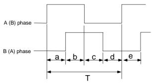
a. b. c. d. e: A phase or B phase rising edge (falling edge) phase difference =  $T/4 \pm T/10$ T: A or B phase cycle (Min. 10µs)
