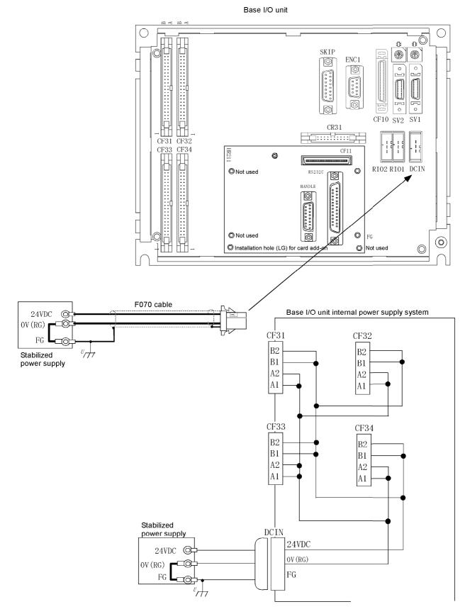
(Note) A 24VDC power supply input is required for both the sink type and source type.
