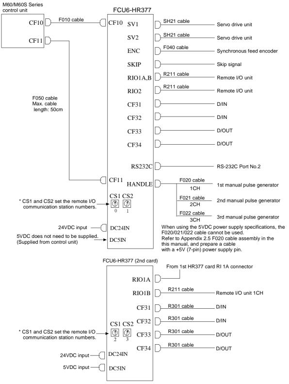
\* When using two FCU6-HR377 cards, the 5VDC for the second card must be supplied from an external source as it is not supplied from the control unit.
