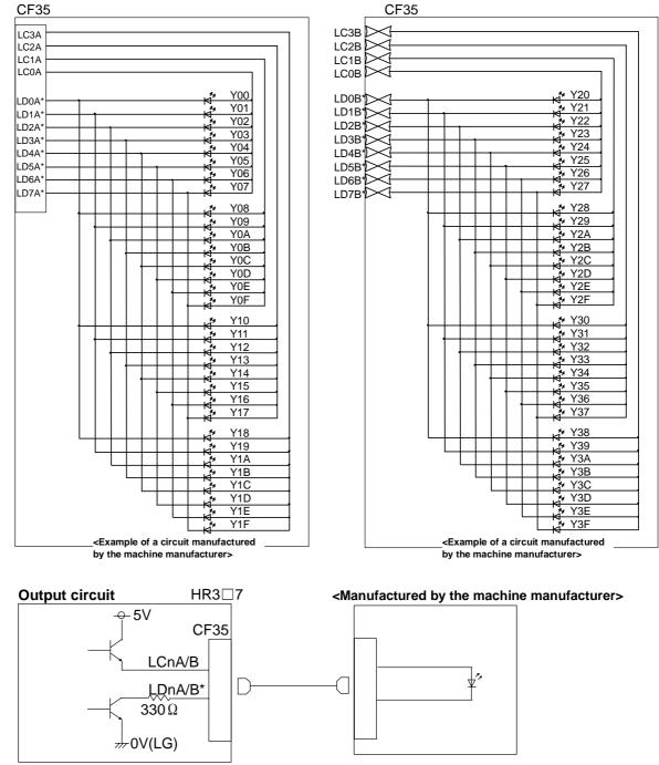
The common signals are changed over with scan output as shown in the following drawing. The LED outputs data, and lights only when the common signal is HIGH. The common signal changes to 4 signals in succession, and lights once every 5.84ms for 1.46ms only. The scan output is a 5V system.
