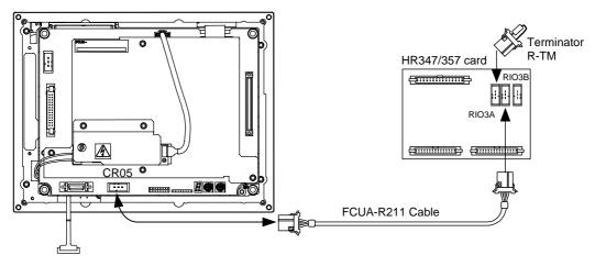
Refer to the explanation on each I/O item for details on setting the number of stations, etc. When connecting the remote I/O, always connect a terminator (R-TM) to the final station. Refer to the "PLC Interface Manual" for details on the interface assignments.
