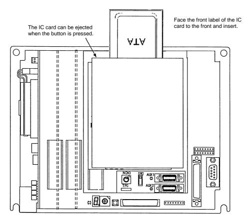
View of control unit lid side with cover removed
