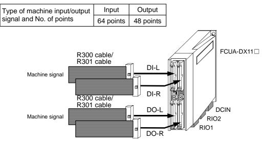
The remote I/O unit cable types include the R300 and R301 types. The R300 cable has one end cut off, and the R301 cable is used for connection to the IDEC IZUMI Corporation terminal block BX1F-T40A<sup>(Note 1)</sup>. The R300-3M and R301-3M cables are available. If a cable longer than 3m is required, use the CN300 and CS301 connector set.
