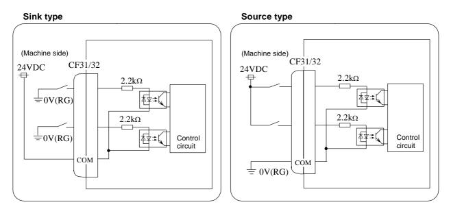
**Input conditions** Use the input signals within the range of the following conditions.
