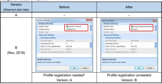
\* When using version A on GX Works3, Profile (for MELSEC iQ-R series Energy Measuring Module (RE81WH) profile) registration is needed
