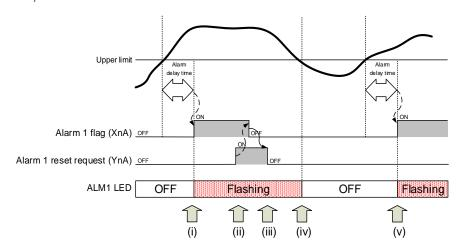
Figure 3.4.4-5 Procedure for resetting Alarm 1 flag (alarm reset method = "Self-reset")
