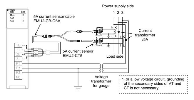
Figure 6.3.3-1 In the case of Three-phase 3-wire system (with the voltage transformer for gauge/current transformer)
