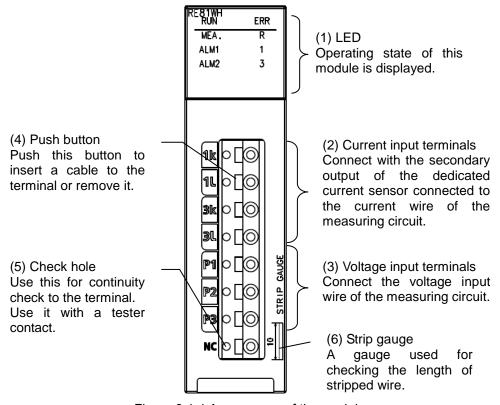
Figure 3.1-1 Appearance of the module
