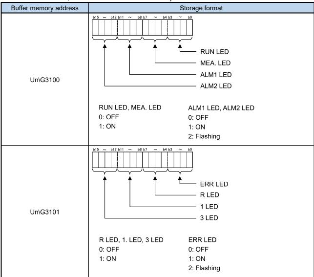
When calculated value is low, "MEA"LED, "R"LED, "1"LED and "3"LED are looked like flashing.
