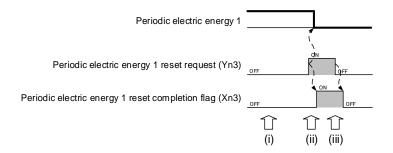
Figure 3.4.2-2 How to reset the periodic electric energy 1
