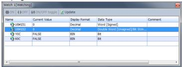
(e) Setting the [Integrated value setting target] (Un\G51) and [Integrated value setting value] (Un\G52, 53).
