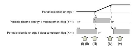
Figure 3.4.2-1 Basic procedure of measuring the periodic electric energy 1
