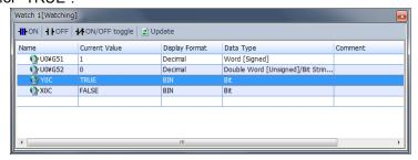
(g) When the settings of [Integrated value setting target] (Un\G51) and [Integrated value setting value] (Un\G52, 53) are reflected, [XnC] changes for "TRUE".
