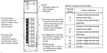
Check the stripping length using the strip gauge of this module.
