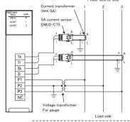
\*For a low voltage circuit, grounding of the secondary sides of VT and CT is not necessary. 0/100/250/400/600) **بال**
