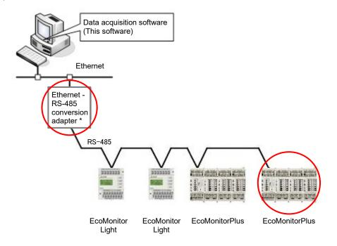
O : Devices that need the connection of a termination resistor
