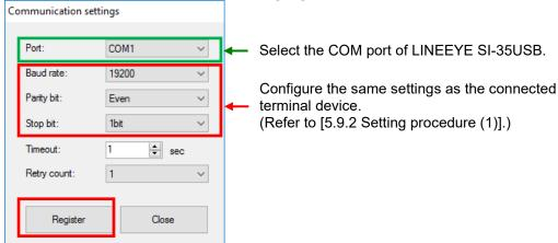
\*How to confirmation the COM port of LINEEYE SI-35USB point the upper-right corner of the screen, move the mouse pointer down, and then click Search, enter Device Manager in the search box, and then click Device Manager.
