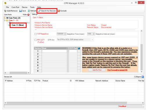
(u) The search result is displayed in Device List.Double-click the IP address of LINEEYE SI-65 from the search result and assign to the COM port.
