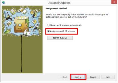
(d) Enter an IP address you want to set to LINEEYE SI-65 and click [Next] button. \*Set an IP address connectable to the PC.
