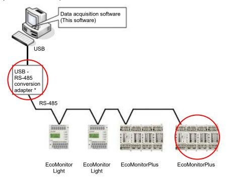
: Devices that need the connection of a termination resistor
