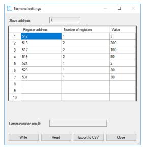
(c) If you want to display the setting of the terminal, input the Register address and Number of registers you want to read as below, and then press [Read] button. For the input value, refer to the MODBUS equipment user's manual.
