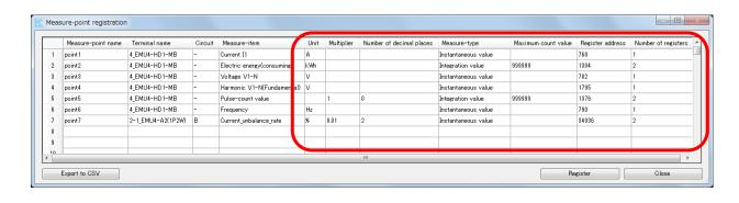
(e) After input of measured item, press [Register] button to complete registration.
