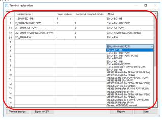
(c) To end the terminal registration, press [Register] button to register the terminals and then press [Close] button.
