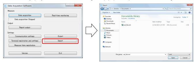
Select setting file (xml file) and open it to start import, and then the setting (Communication setting, Terminal registration / setting, Measure-item registration) is changed.
