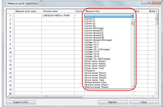
(d) After choosing Measure-item, input Measure-point name. Unit, Measure-type, Maximum count value, Register address and Number of registers are input automatically. You do not need to input anything to blanks except for Measure-point name.
