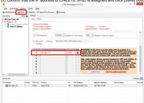
(v) Confirm that the IP address of LINEEYE SI-65 is assigned and click [Save] button.
