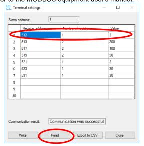
(d)If you want to change the setting of the terminal in this window, input the Register address and Number of registers you want to write as below, and then press [Write] button. For the input value, refer to the MODBUS equipment user's manual.
