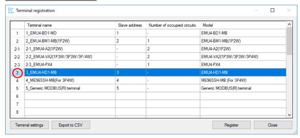
\* If you want to delete the registered terminal, select the number of the terminal you want to delete at the left hand position of the display, and press DELETE key on the keyboard to delete it.
