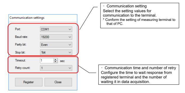
\* Port : COM port to be used in serial communication for MODBUS communication.
