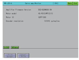
Displays the servo amplifier software number and servo motor information (model name, ID and encoder resolution).
