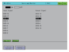
• Displays a list of the ON/OFF status of the external I/O signals of the servo amplifier.
