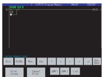
After searching for coil M120 that is in the OFF state, "M669" and "M23" are displayed as devices that are not conductive.
