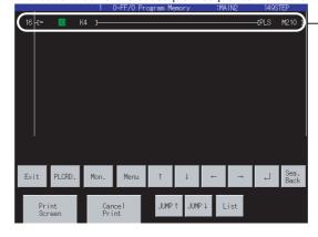
(3) Indirect specification device read Indirect specification devices (index register (Z)) cannot be specified and read when the MELSEC-Q/QnA ladder monitor is executed.
