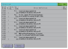
Displays the history of errors that occurred on and after the leading edge of PLC ready (M2000).
