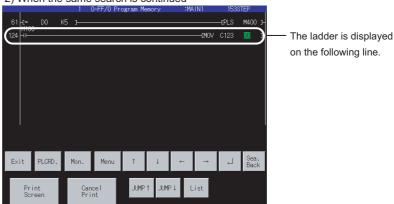
When searching multiple files with the MELSEC-Q/QnA ladder monitor, displaying the ladder block of the subsequent sequence file clears the previous display.
