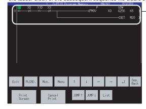
Coil search displays the ladder block that contains a specified coil.
