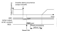
Checking the inverter operating status by the inverter operation ready completion signal
