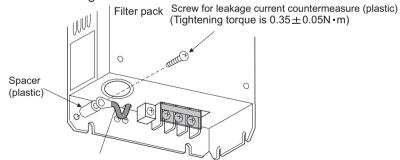
Earth (Ground) cable for capacitive filter
