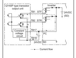
Source logic type Use terminal SD as a common terminal, and perform wiring as shown below. (Do not connect terminal PC of the inverter with terminal +24V of the external power supply. When using terminals PC-SD as a 24VDC power supply, do not install an external power supply in parallel with the inverter. Doing so may cause a malfunction in the inverter due to undesirable currents.)
