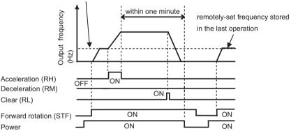
•When the remotely-set frequency is cleared by turning on the RL (clear) signal after turn off (on) of both the RH and RM signals, the inverter operates at the speed in the remotely-set frequency cleared state if power is reapplied after one minute has elapsed since turn off (on) of both the RH and RM signals.
