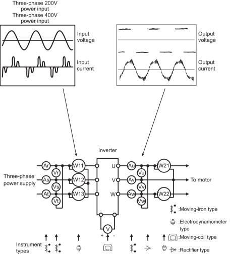
**Examples of Measuring Points and Instruments**
