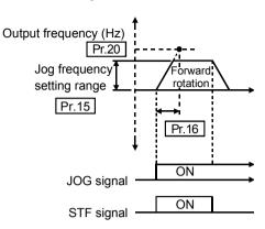
• Set the frequency and acceleration/deceleration time for jog operation.
