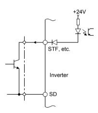
External signal input using transistor
