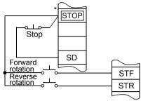
(Wiring example for sink logic)
