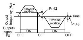
This function is effective for switching the timing of electromagnetic brake operation between forward rotation (rise) and reverse rotation (fall) during vertical lift operation, etc.
