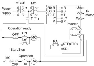
Inverter Start/Stop Circuit Example (with filter pack)
