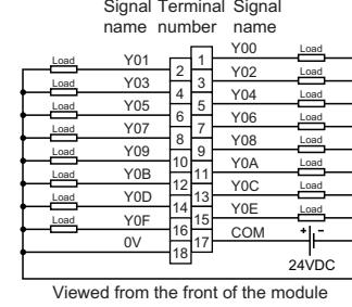
For the wiring diagram to use the module in SIL2 mode, refer to the MELSEC iQ-R I/O Module (With Diagnostic Functions) User's Manual (Application).
