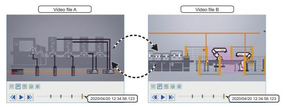
A log marker added to a video file in Video Verification Tool can be applied to a recording file or data logging file in GX Works3 and GX LogViewer. ( Page 22 GX Works3, Page 22 GX LogViewer)
