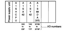
(2) D/A Conversion Module I/O Signals
