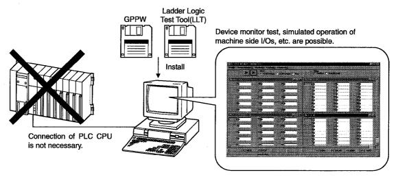
A sequence program created with GPPW can be debugged by writing it to the ladder logic test tool (LLT).
