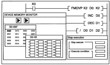
8) Double-click on X0 in the DEVICE MEMORY MONITOR window and force X0 ON to run the program above.
