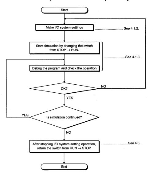
The flowchart shows the procedure to execute the I/O system setting functions.
