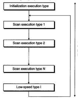
(Assume 1 scan uses 100 ms, then execution of 5 scans = 500 ms. Changing of a reference time is possible by changing the constant scan time (See 2.4.1, item (1)).
