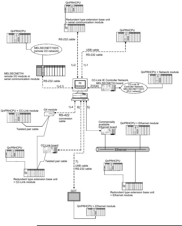
(6) Connecting to a Redundant CPU in the Debug Mode (QnPRHCPU)
