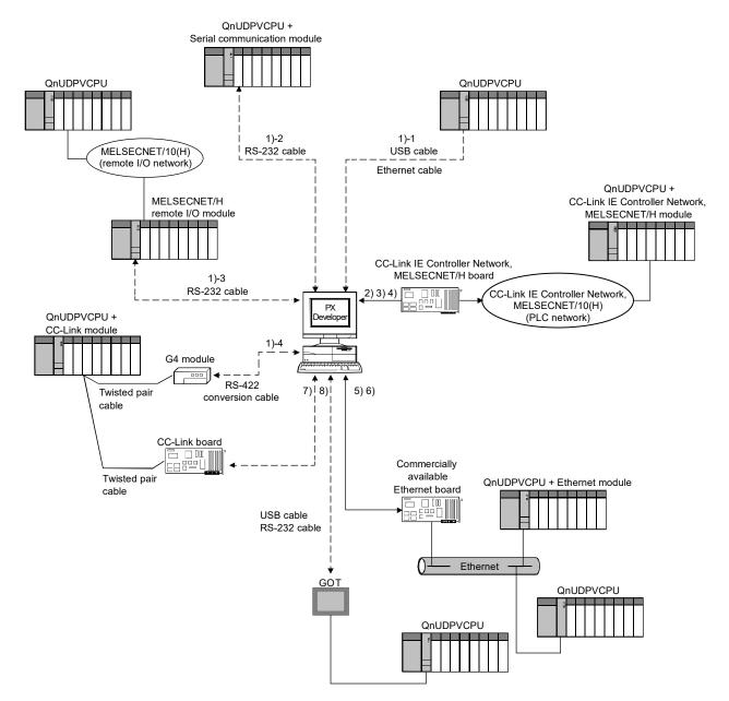
(4) Connecting to a Universal model process CPU(QnUDPVCPU)
