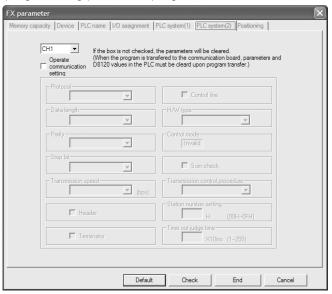
When the PLC type of the project is the FX<sub>3G</sub> or FX<sub>3U(C)</sub>, the channel setting (CH1/CH2) combo box is displayed. Select "CH1" to confirm the setting.
