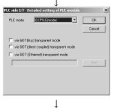
4. When connecting a GOT and a programmable controller, set the following according to the connection method, and then click OK button.
