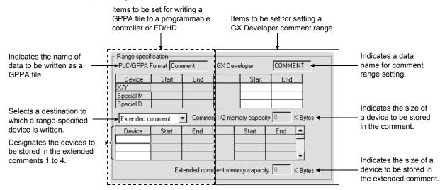
If the starting and end positions of a range are designated in GX Developer files, they are reflected in the PLC /GPPA table.
