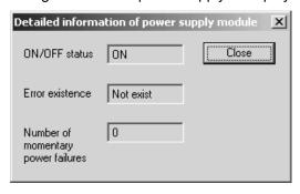
In the case of multiple CPU system, the information can be displayed only when specifying the connected destination as No.1 CPU. To check the latest status, close this screen and then open it again.
