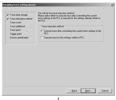
Select whether trace will be executed on the conditions set using GX Developer or the settings for programmable controller.
