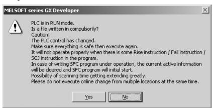
Click the Yes button to write the data specified on the Write to PLC screen to the programmable controller.
