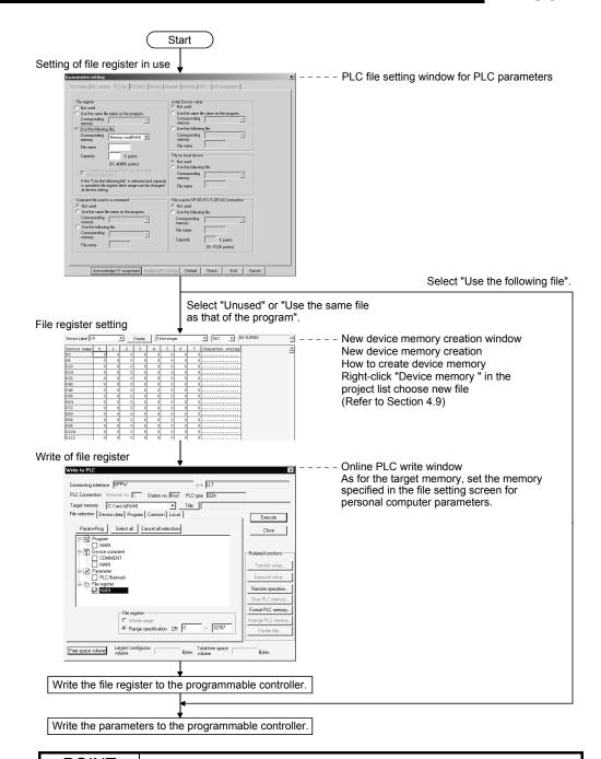
When creating and writing a new file register name that is the same as the file register name written to the programmable controller, delete the existing file register from the programmable controller.
