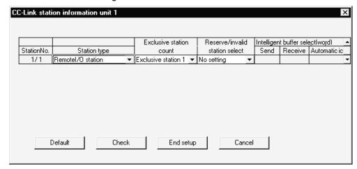
After setting the CC-Link parameters, write them to the programmable controller.
