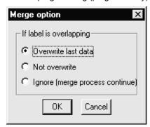
If the data to be merged include the data which exceeds the device range of the merge destination CPU, the comment data in the excess area is deleted.
