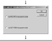
Check the "via GOT-F900 transparent mode" checkbox, and click the OK button. (This is not necessary for models other than FX3G, FX3U, FX3UcCPU.)
