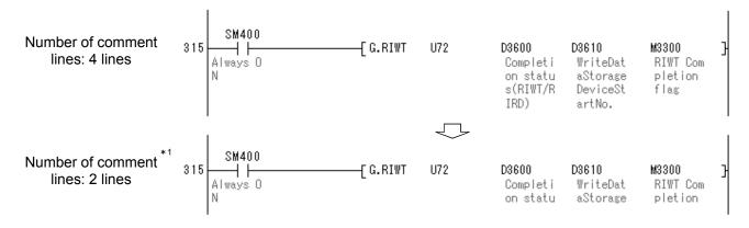
\*1: The lines after the set number of comment lines (For example, 3 and 4 lines on the diagram above) are not displayed.
