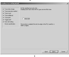
This screen is for Universal model QCPU only. Set to auto start the sampling trace when the state of CPU turns to RUN state.
