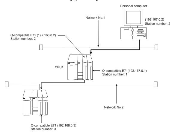
Procedure for communications via Q-compatible E71
