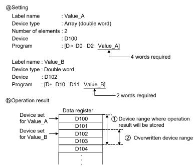
In the above case, make setting to assign the device of the label (Value\_B) to D104.
