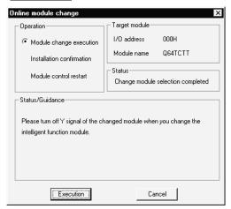
Depending on the faulty condition of the module to be changed, the type of the module may not be acquired. In that case, "Unknown" appears in the Target module name display field.
