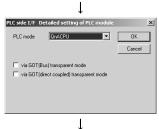
4. When connecting GOT and programmable controller via bus connection, select "Via GOT(Bus) transparent mode", when directly connecting them, select, "Via GOT(direct coupled) transparent mode" by checking the check box, and then click OK button.
