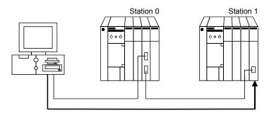
(1) Computer link module switch settings Station 0 (Connect GX Developer to the RS-232 connector of the computer link module.)
