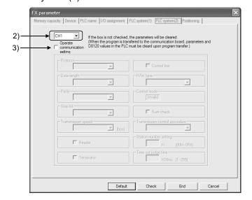
When the PLC type of the project is the FX3G or FX3U(C), the channel specification (CH1/CH2) combo box is displayed.
