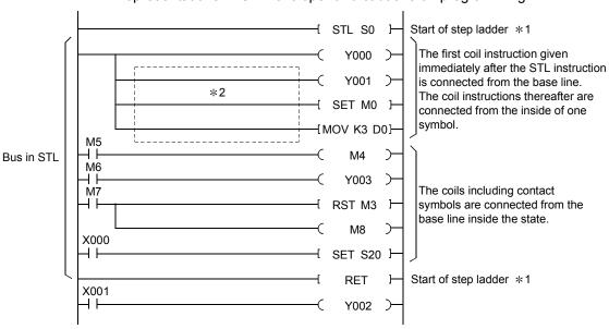
Though the FX series programming material gives descriptions using the above conventional representations, they must be given in a GPPW-specific style when the step ladder instructions are input by GX Developer.
