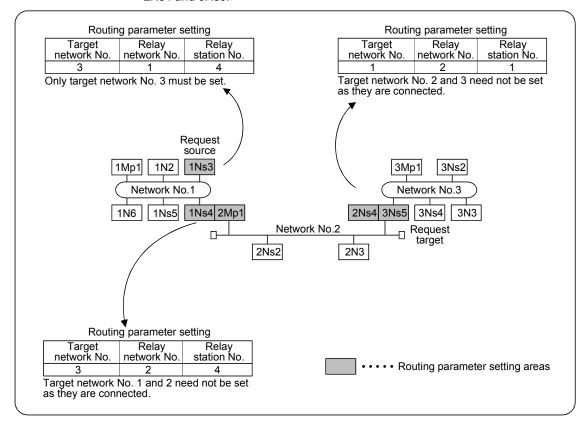
(2) Up to 16 "Target network No.s" can be set to the programmable controller. 64 different network No.s allow the own station to be a request source or other stations to be accessed via the own station.
