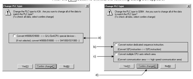
a) Check this check box when making conversion between the M9000/ D9000 range and the Q/L/QnACPU special devices.
