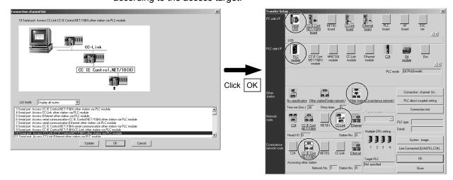
Clicking the OK button automatically sets the connection channel (areas enclosed by circles) on the Connection Setup screen.
