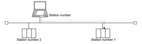
A PING test can be made only within the same segment.
