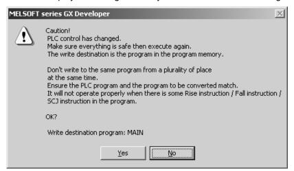
Click the Yes button to write the modified program to the programmable controller.
