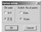
Bit & word format (for FX series X, Y monitor)
