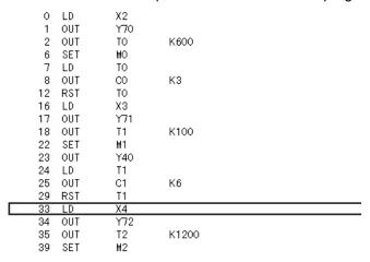
3. Enter an instruction to be inserted or added or device (LD M10), then the list input dialog box is displayed with the entered data being displayed in the device instruction text box.
