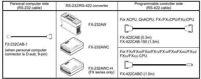
How to identify compatibility of the F2-232CAB and F2-232CAB-1 cables with the ACPU and QnACPU
