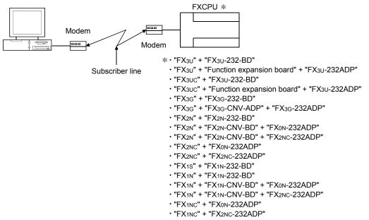
In the FX3UC series, only the FX3UC-32MT-LT and FX3UC-32MT-LT-2 are connectable.
