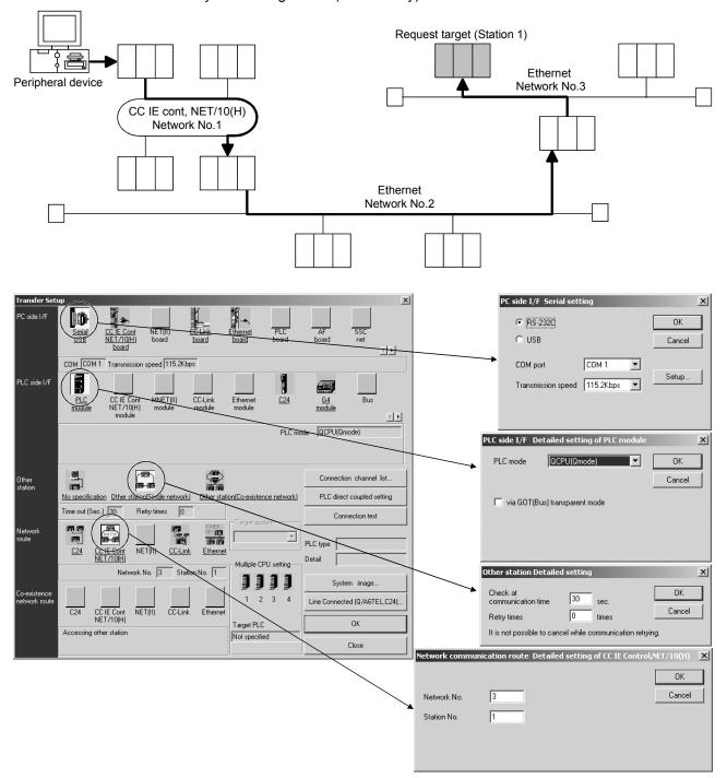
For access to the other station or multilevel system, not only the Connection Setup but also the routing parameters should be set to enable communications.
