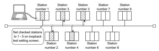
A loopback test can be made only on the Ethernet modules of the loopback test target network No.
