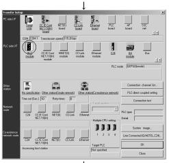
3. Double-click "PLC module" in the PLC side I/F.
