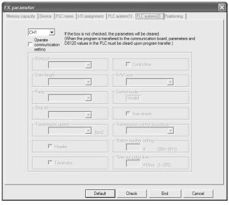
When the PLC type of the project is the FX<sub>3U(C)</sub>, the channel specification (CH1/CH2) combo box is displayed. Select "CH1" to confirm the setting.
