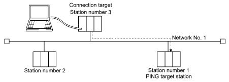
A PING test can be made only on the Ethernet module in the same segment as that of the PING test target station.
