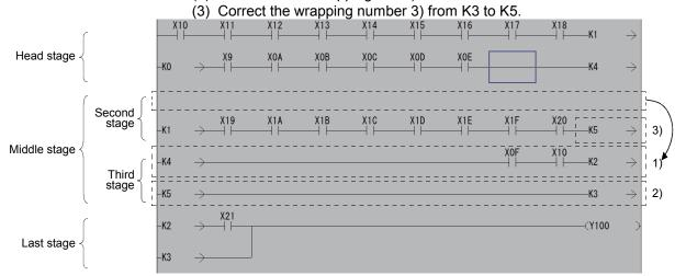
11. When an overwrite contact or coil extends over multiple contacts, the circuit cannot be edited in write (overwrite) mode.
