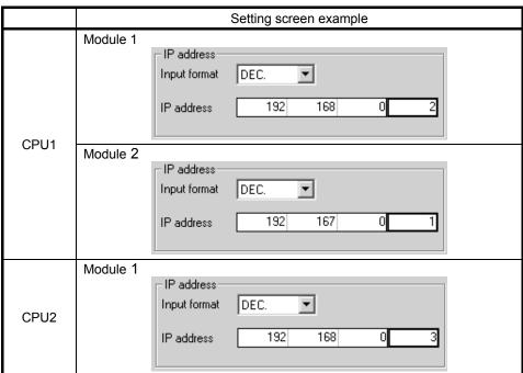
To make communications with GX Developer, ask the person in charge of the network about the IP address setting to confirm, and set the IP address. Since "any" values may be set to the other items, set them according to the specifications of the other node and application connected to the Q seriescompatible E71.
