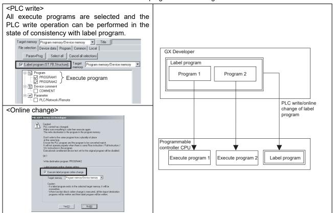
PLC write/online change of execute programs must be performed with label programs because program inconsistency occurs when PLC write/online change of only execute program is performed to a programmable controller CPU.
