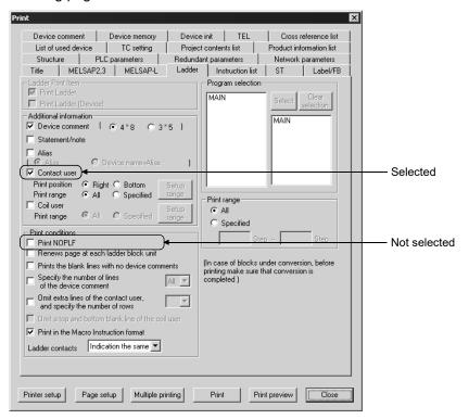
If there are two or more lines of contact user under the above settings, pages will be fed in the middle of the lines. Pages will not be fed in the middle of the ladder and the coil using data.
