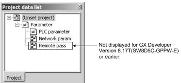
(b) When the project is saved, its set remote password is not deleted. (Saved unchanged)
