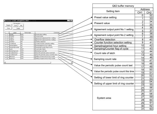
5. Click on [Project] tab to display "Local variable setting" screen and set the local label of program. After the above setting is completed, execute [Convert/Compile].
