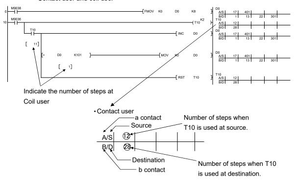
Only the locations of contact/coil users which are used in the same program are displayed.
