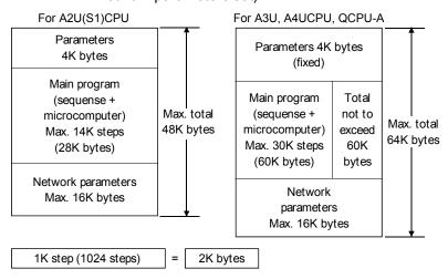
(b) Main program + subprogram capacity Write A3U/A4UCPU, QCPU (A mode) subprograms together with the main program. It is not possible to write a subprogram by itself. When writing a main program + subprogram, the main program capacity set in the PLC parameters, the automatically added parameters (fixed at 4K bytes), and the subprogram capacity, are written to the ROM. The subprogram capacity is automatically set at 64K bytes per subprogram.
