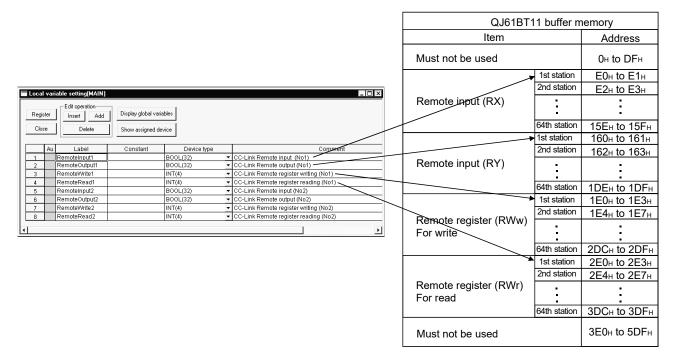
2. Set the array in a sequence program as shown below.
