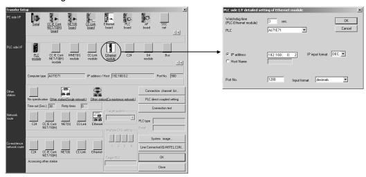
PLC side I/F detailed setting of Ethernet module
