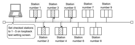
A loopback test can be made on the other network No.
