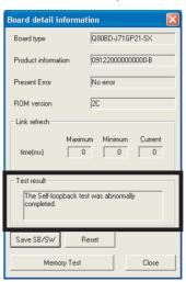
If the test completes abnormally, replace the optical fiber cable and execute the test
