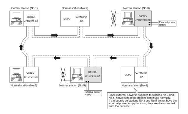
When CC-Link IE Controller Network boards without the external power supply function are installed to station number 3 and 5, and if personal computers of these stations are powered off, station number 3, 4, and 5 will be disconnected from the network.
