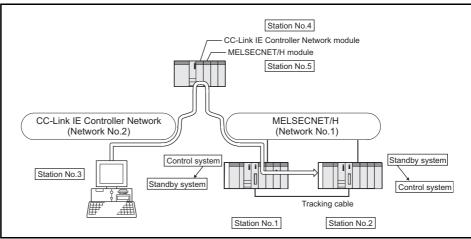
To check which system in the Redundant CPU system is being accessed by the CC-Link IE Controller Network board, create a program to monitor the following special relays.
