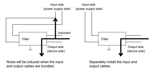
• Ground the ground terminal of the noise filter to the ground point of the control panel with the shortest cable possible (approximately 10 cm).
