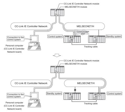
Figure 1 Path switching example 1
