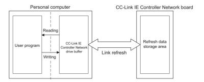
\*1: Separation is a condition that link data with double words (32 bits), such as the current value of the positioning module, are separated to new data and old data in units of one word (16 bits) due to the refresh timing of cyclic transmission.
