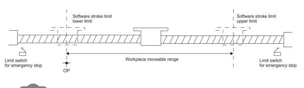
In general, the  $\ensuremath{\mathsf{OP}}$  is set at the lower limit or upper limit of the software stroke.
