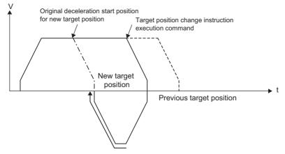
• If the workpiece is decelerating when the execution command for Target position change instruction (IPTPCHG1(P)) is established, the axis decelerates to a stop and then positions itself to the new target position.
