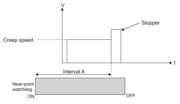
• When starting position is in interval B (between the near-point dog OFF position and stopper) in the figure below, no near-point dog is detected and thus the axis may collide with the stopper at the OPR speed.
