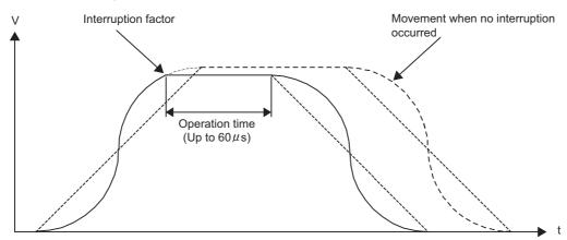
Since pulses are output during constant-speed operation, the positioning address may be reached during deceleration. In this case, the axis stops immediately upon reaching the positioning address.
