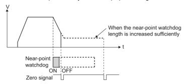
For the method to calculate the distance from the near-point dog ON position to OP, refer to F Page 69, Section 7.6 (8).
