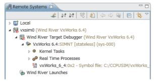
9. When the connection to the simulator is established, the tree to the left is displayed on the "Remote Systems" window and the "Target Console" screen appears.
