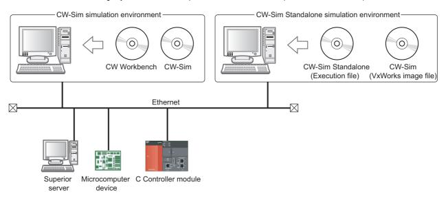
Programs running on the simulator can be interlocked with superior server, microcomputer device, and C Controller module via Ethernet.
