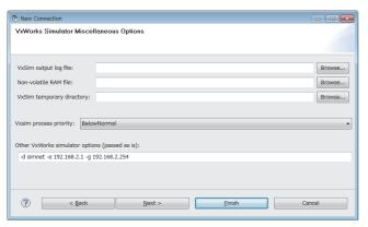
7. Set the IP address and default gateway of the virtual network for "Other VxWorks simulator options".
