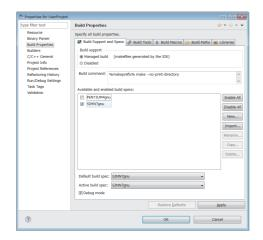
2. Select [Build Properties] from the tree view to the left on the window, and click the <<Build Support and Specs>> tab.
