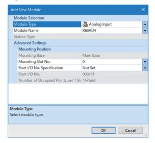
**5.** Set the window as follows to add the module label of the A/D converter module.
