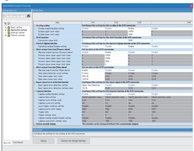
**8.** Write the set parameters to the CPU module on the master station. Then, reset the CPU module or power off and on the system.
