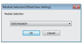
**2.** Select the target module for the offset/gain setting, and click [OK] button.
