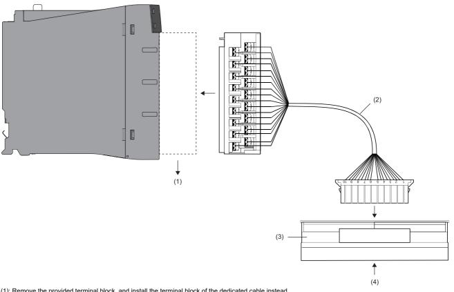
(1): Remove the provided terminal block, and install the terminal block of the dedicated cable instead.
