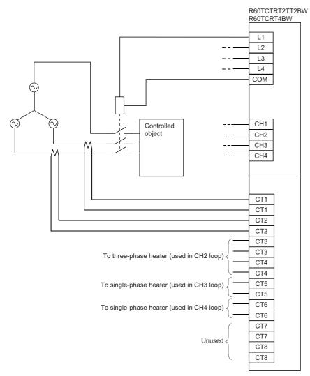
The disconnection of the three-phase heater is detected by measuring the currents of two of the three cables. In the above wiring example, set "CT input channel assignment setting" of "CT setting" as indicated below.
