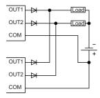
· When providing another circuit in parallel with a transistor output module
