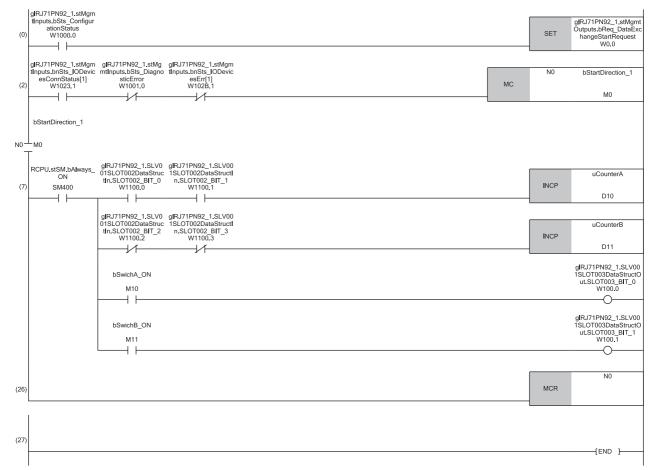
(7) Program to process I/O data to IO device 1
