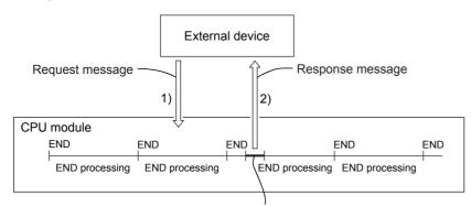
Processing for a command from the external device
