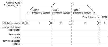
• If pbi\_bTableExeMethod (Table execution method) is off, stepping operation of the multiple table operation (DRVTBL) instruction is performed together with an added function for automatic table transfer.
