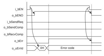
Module error (Serial communication sending error) <ch1 example>
