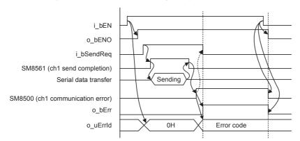
Module error (Serial communication receiving error) <ch1 example>
