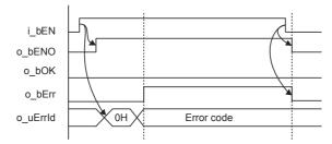
Module error (Serial communication error) <ch1 example>
