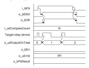
In the case of "o\_udOutputOnTotal (Integration value of number of relay ON times) > i\_udCompareCount (Number of comparisons)"
