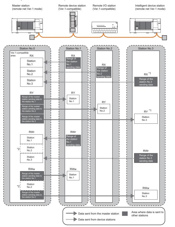
\*1 The last 16 bits in RX, RY cannot be used when using the master/intelligent device module as the intelligent device station.
