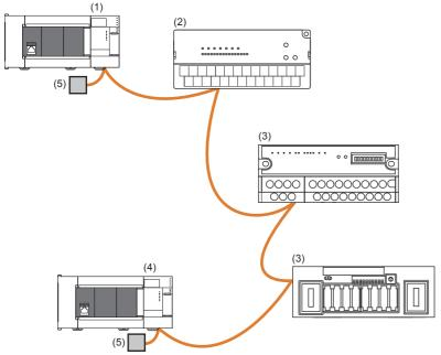
The CC-Link version and the number of device stations that can be connected vary depending on the mode of the master/ intelligent device module. (EP Page 22 Maximum Number of Connectable Modules (when operating as a master station)) 5
