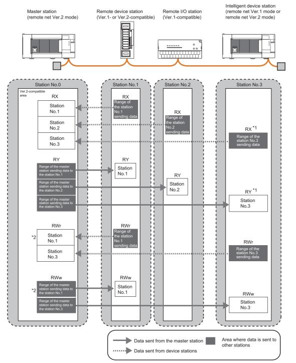
\*1 The last 16 bits in RX, RY cannot be used when using the master/intelligent device module as the intelligent device station.
