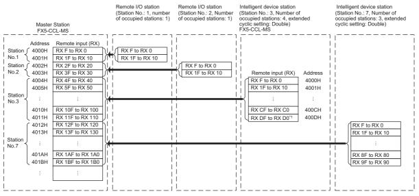
\*1 The last 2 bits of RX cannot be used when using the master/intelligent device module as the intelligent device station.
