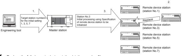
**1.** Replace the failed remote device station (station number 3).
