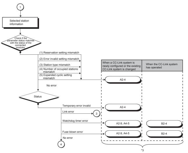
\*3 The item corresponds to the number of the check item for when a device station is disconnected. Refer to the corresponding check item and take the action. ( 🖙 Page 128 When a device station is disconnected)
