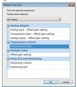
1. Select "Temperature trace" in "Temperature Control Module" and click the [OK] button.
