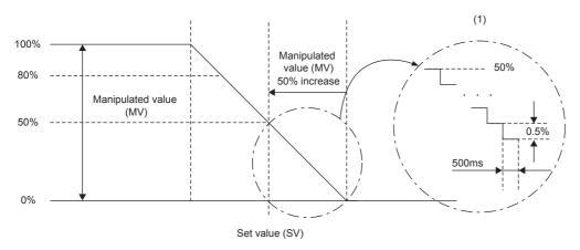
(1) When 'CH1 Output change ratio limiter' (Un\G510) has been set to 10 (1.0%/s)
