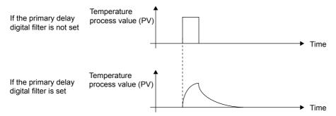
Set the time for the temperature process value (PV) to change by 63.3% in the primary delay digital filter.
