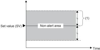
(1) 'CH1 Loop disconnection detection dead band' (Un\G538) (this band has the set value (SV) at the center)\*1
