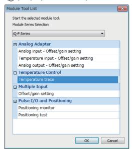
**1.** Select "Temperature trace" in "Temperature Control Module" and click the [OK] button.
