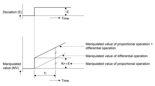
An integral action is used as a PI action in combination with a proportional action, or a PID action in combination with a proportional action and a derivative action. An integral action cannot be used by itself.
