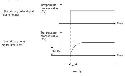
(1) 'CH1 Primary delay digital filter setting' (Un\G563)
