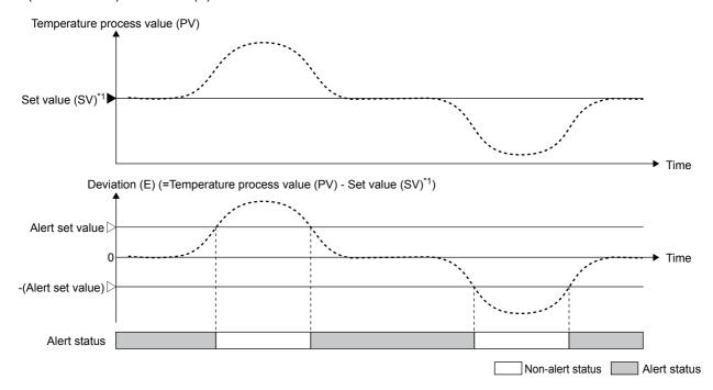
\*1 Depending on the alert mode setting, this value becomes the set value or the monitored value. The setting range of the alert set value is (-(Full scale of the input range)) to the full scale of the input range. (Fig. 8) Page 54 Setting the set value (SV) and the setting change rate limiter)
