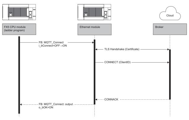
To use TLS connection, the MQTT client performs a TLS handshake before sending the CONNECT command. During the handshake, the client and broker exchange their certificates with each other. The client and broker must be configured in advance to trust each other's certificates.
