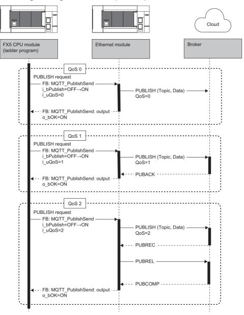
To send a message to a broker, the MQTT client (Ethernet module) sends the PUBLISH command to a broker. Communication with the broker is performed according to QoS. The following three QoS levels exist.
