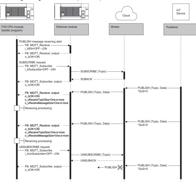
As a subscriber, the MQTT client uses FB: MQTT\_Subscribe to send a broker the SUBSCRIBE command to request a topic to subscribe. The broker returns the SUBACK command to the subscriber. When the requested topic matches a topic in the PUBLISH command received from publishers, the broker uses the PUBLISH command to send the topic name and data to the subscriber.
