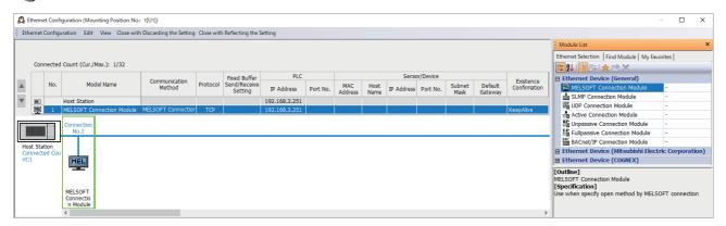
Drag and drop an "Ethernet Device" in the "Module List" to the left side of the screen, and set the following items. The setting items vary depending on the "Ethernet Device" and "Communication Method".
