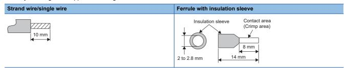
Check the shape of the wire insertion opening with the following chart, and use the smaller wire ferrule than the described size. Also, insert the wire with care so that the wire ferrule is in proper orientation. Failure to do so may cause the bite of the terminal and the damage of the terminal block.
