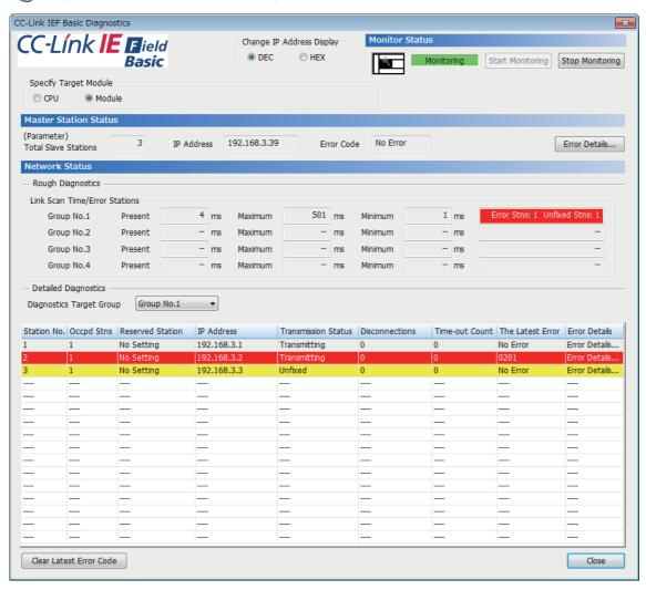
The status of the master station is checked in "Master Station Status".
