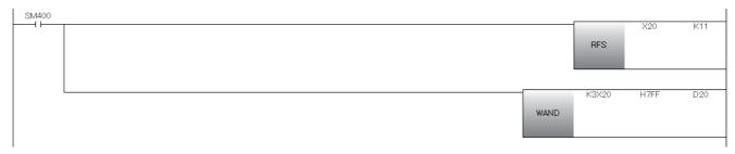
3. When the gray code is output from the absolute encoder, the gray code data is converted to BIN 16-bit data.
