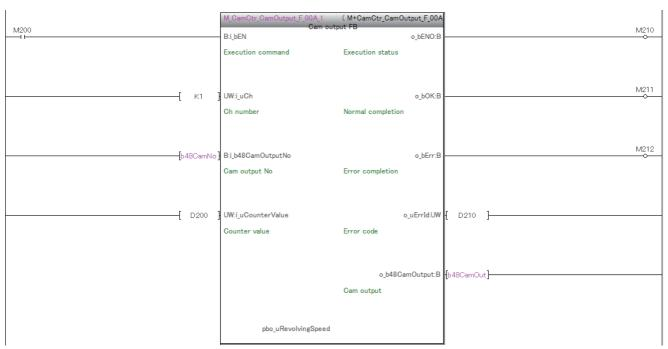
7. Reflect the cam output status set by the cam output FB to Y device to refresh it.
