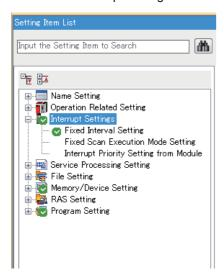
3. Set the fixed cycle interval of I31 in "Interrupt Setting from Internal Timer" to "1 ms".
