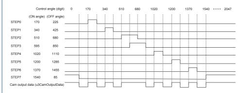
When the cam output data is not set, the ON angle and OFF angle of STEP 0 to STEP 7 become 0. To prevent the ON output without setting, when the ON angle and OFF angle are the same in a STEP, the corresponding angle outputs OFF. When the ON angle and OFF angle are the same in different STEPs (for example, when STEP 1 ON angle = STEP 2 OFF angle), the corresponding angle outputs ON.
