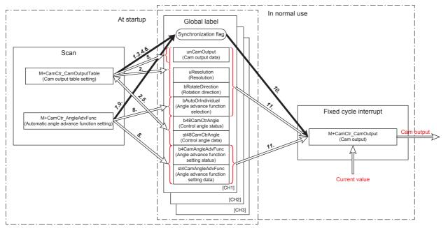
At the startup, use M+CamCtr\_CamOutputTable (Cam output table setting) and M+CamCtr\_AngleAdvFunc (Automatic angle advance function setting) and set each cam output data of the global label.
