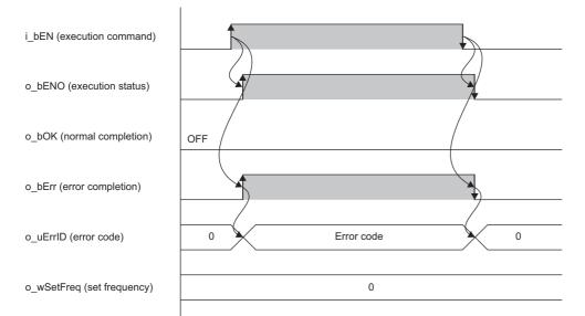
When an error occurs while the FB is operating (when the first motor is controlled and the setting value of the first motor set frequency is out of the setting range)
