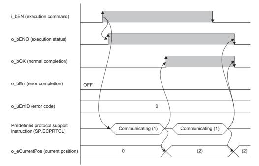
(1) While the FB is being executed, the predefined protocol support instruction (SP.ECPRTCL) is executed at any time.(2) A value obtained from a distance meter
