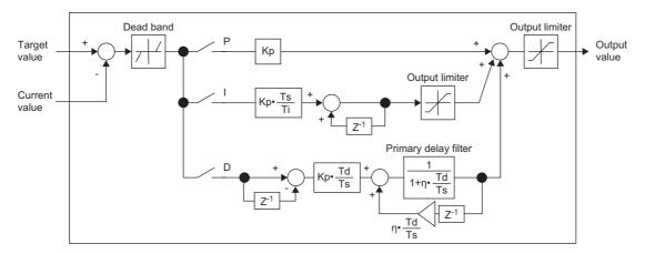
P: Proportional operation, I: Integral operation, D: Differential operation
