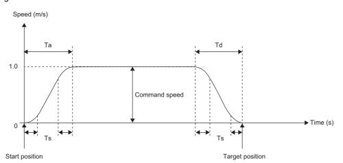
The acceleration rate and deceleration rate and the acceleration jerk and deceleration jerk can be calculated from the acceleration/deceleration reference speed, the acceleration time and deceleration time, and the S-curve time.
