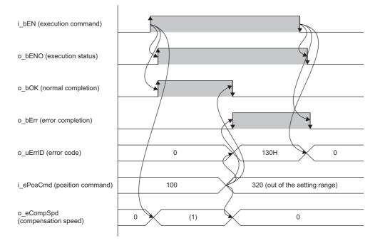
(1) Compensation speed [m/s]: While the FB is being executed, a calculated value is output every scan.
