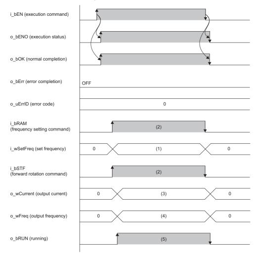
(1) Set frequency [0.01 Hz increments]: While the FB is being executed, the value is written to the inverter every scan.
