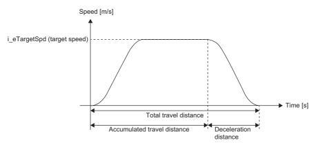
To calculate the deceleration distance, call M+AWH\_DecDistance\_F (deceleration distance calculation) from this FB.
