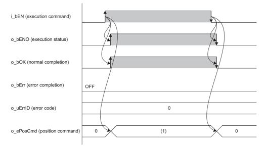
(1) Position command [m] after anti-sway control calculation: While the FB is being executed, the calculated value is output every scan.
