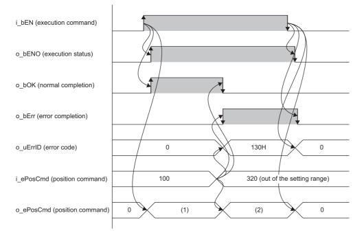
(1) Position command [m] after anti-sway control calculation: While the FB is being executed, the calculated value is output every scan. (2) i\_ePosCmd (position command) [m]
