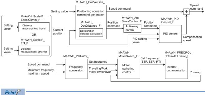
Use M+AWH\_AntiSwayControl\_F (anti-sway control) and M+AWH\_MotorSwitch\_F (motor switching control) according to the user's system and the expected operation.
