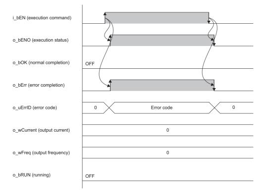
When an error occurs while the FB is operating (when the setting value of the set frequency is out of the setting range)
