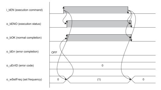
(1) Set frequency [0.01 Hz increments]: While the FB is being executed, a calculated value is output every scan.
