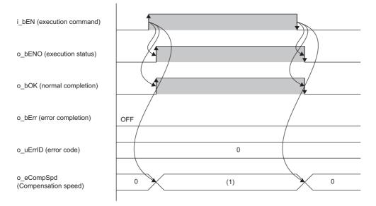
(1) Compensation speed [m/s]: While the FB is being executed, a calculated value is output every scan.
