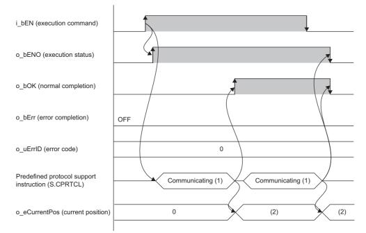
(1) While the FB is being executed, the predefined protocol support instruction (S.CPRTCL) is executed at any time.(2) A value obtained from a distance meter
