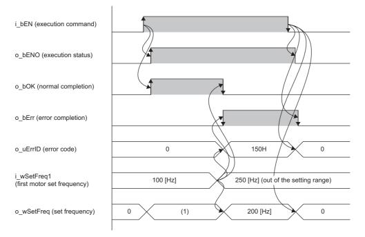
(1) First motor set frequency: While the FB is being executed, the calculated value is output every scan.
