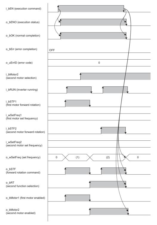
(1) First motor set frequency: While the FB is being executed, the calculated value is output every scan.
