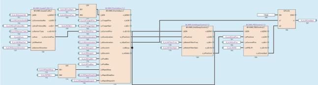
(2) Speed command  $\rightarrow$  Frequency conversion to inverter communication
