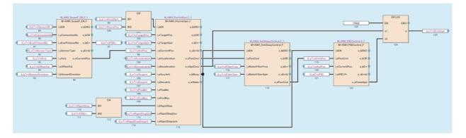
(2) Speed command  $\rightarrow$  Frequency conversion, travel/fork motor switching control, inverter communication
