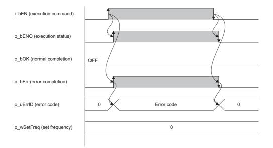
When an error occurs while the FB is operating (when the absolute value of the speed command exceeds the maximum speed)
