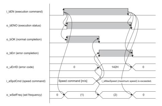
(1) Set frequency [0.01 Hz increments]: While the FB is being executed, a calculated value is output every scan.
