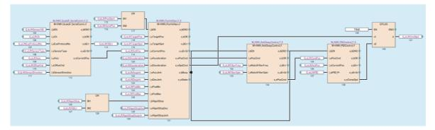
(2) Speed command  $\rightarrow$  Frequency conversion to inverter communication
