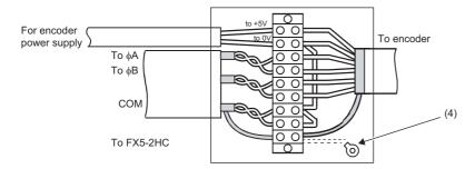
(4) Between the encoder and the shielded twisted pair cable, connect their shield wire together in the relay box. If the shield wire of the encoder to be used is not grounded in the encoder, ground it in the relay box as the dotted line shows.
