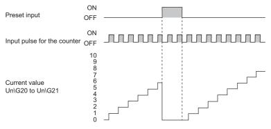
The preset is constantly executed while the preset input is ON.
