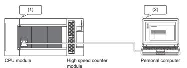
The CPU module collects and saves information on events that occurred in the high-speed counter module.
