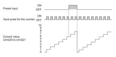
The preset is executed when the preset input changes  $ON \rightarrow OFF$ .
