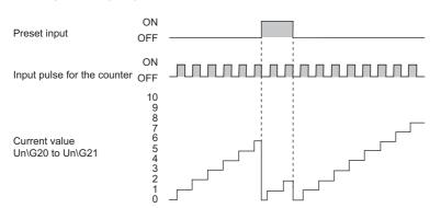
The preset is executed when the preset input changes OFF→ON and when it changes ON→OFF.
