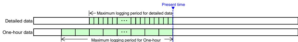
This optional plug-in module stores the data of logging period from current time in the internal memory. Data older than the maximum logging period is erased.
