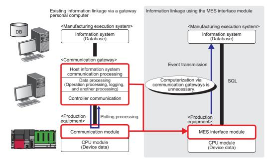
The following describes the overall system configuration when using the MES interface module.
