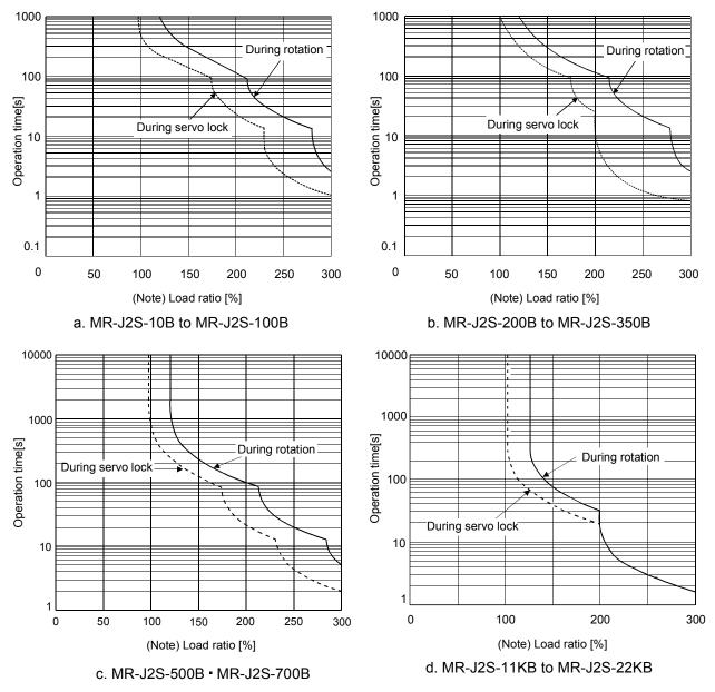
Note. If operation that generates torque more than 100% of the rating is performed with an abnormally high frequency in a servo motor stop status (servo lock status) or in a 30r/min or less low-speed operation status, the servo amplifier may fail even when the electronic thermal relay protection is not activated.
