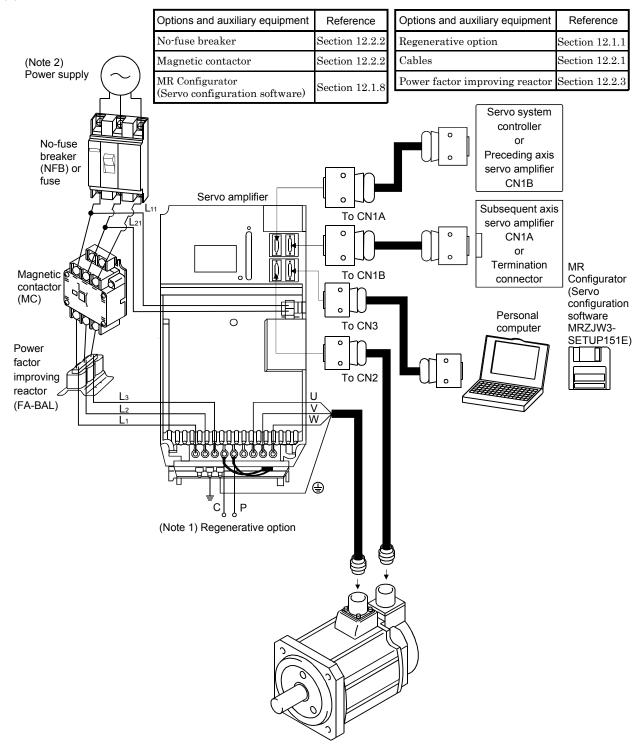
Note 1. When using the regenerative option, remove the lead wires of the built-in regenerative resistor.
