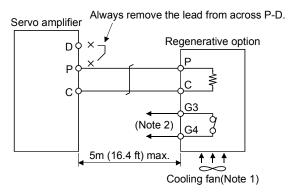
Note 1. When using the MR-RB50, forcibly cool it with a cooling fan (92 × 92, minimum air flow: 1.0m<sup>3</sup>).
