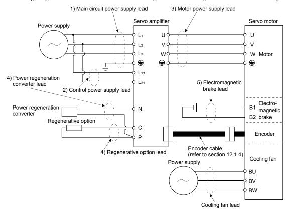
The following table lists wire sizes. The wires used assume that they are 600V vinyl wires and the wiring distance is 30m(98.4ft) max. If the wiring distance is over 30m(98.4ft), choose the wire size in consideration of voltage drop.
