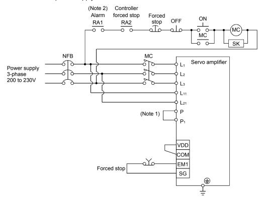
Note 1. Make sure to connect P1-P. (Factory-wired.) When using the power factor improving DC reactor, refer to section 12.2.4.
