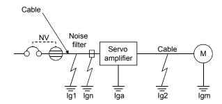
K: Constant considering the harmonic contents Leakage current breaker Mitsubishi Κ Type products NV-SP NV-SW Models provided with harmonic and surge NV-CP 1 reduction techniques NV-CW NV-HW BV-C1 General models NFB 3 NV-L
