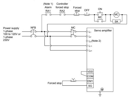
Note 1. Configure up the power supply circuit which switches off the magnetic contactor after detection of alarm occurrence on the controller side.
