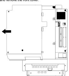
3) Remove the front cover by drawing it in the direction of arrow.
