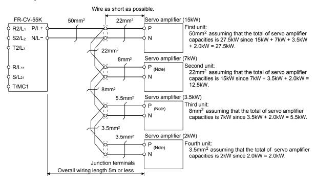
Note. For 7kW or less servo amplifier, always remove the wiring (3.5kW or less: across P-D, 5k • 7kW: across P-C) of built-in regenerative resistor.
