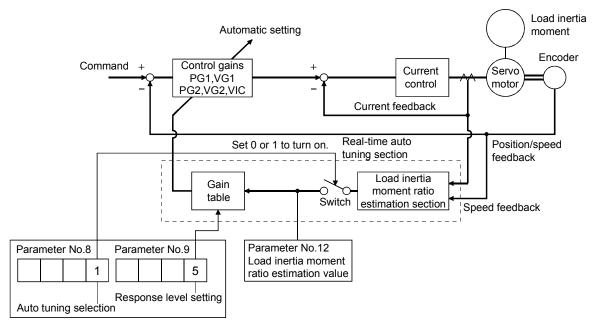
When a servo motor is accelerated/decelerated, the load inertia moment ratio estimation section always estimates the load inertia moment ratio from the current and speed of the servo motor. The results of estimation are written to parameter No. 12 (the ratio of load inertia moment to servo motor). These results can be confirmed on the status display screen of the MR Configurator (servo configuration software) section.
