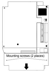
1) Remove the front cover mounting screws (2 places) and remove the front cover.
