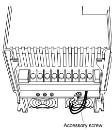
For the MR-RB50 • MR-RB51 install the cooling fan as shown.
