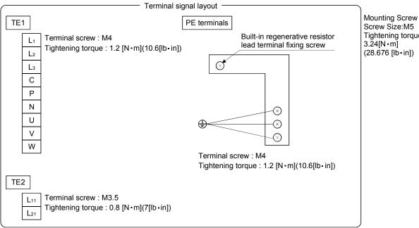
Screw Size:M5 Tightening torque: 3.24[N·m] (28.676 [lb•in])
