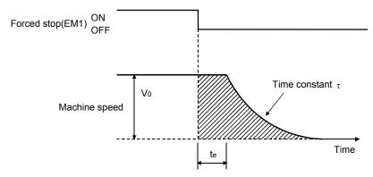
Fig. 11.3 Dynamic brake operation diagram
