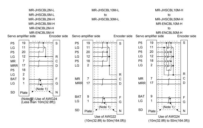
Note 1. This wiring is required for use in the absolute position detection system. This wiring is not needed for use in the incremental system.
