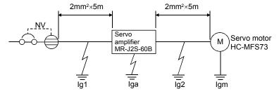
Use a leakage current breaker designed for suppressing harmonics/surges. Find the terms of Equation (12.1) from the diagram.
