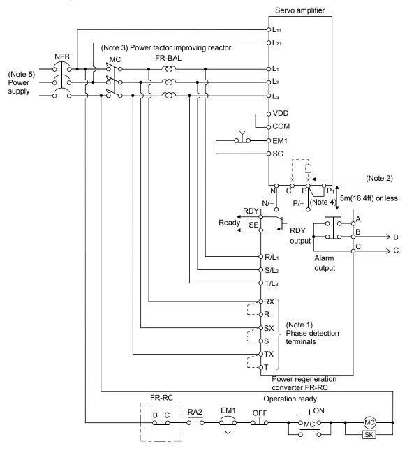
Note 1. When not using the phase detection terminals, fit the jumpers across RX-R, SX-S and TX-T. If the jumpers remain removed, the FR-RC will not operate.
