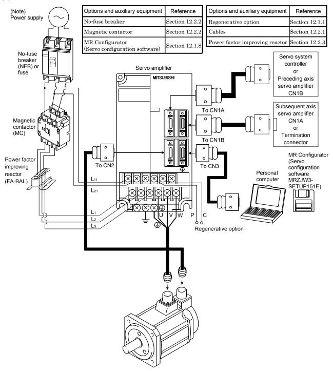
Note. Refer to section 1.3 for the power supply specification.
