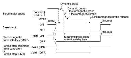
Note. ON: Electromagnetic brake is not activated.
