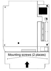
3) Fit the front cover and fix it with the mounting screws (2 places).
