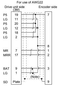
Note. Always make connection for use in an absolute position detection system. This wiring is not needed for use in an incremental system.
