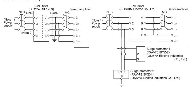
Note 1. For 1-phase 230V power supply, connect the power supply to L<sub>1</sub>, L<sub>2</sub> and leave L<sub>3</sub> open. There is no L<sub>3</sub> for 1-phase 100 to 120V power supply. Refer to section 1.3 for the power supply specification.
