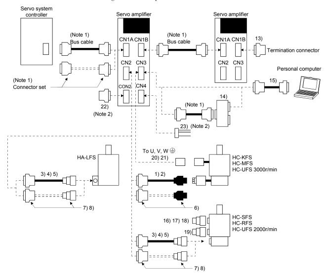
Note 1. The bus cable used with the SSCNET depends on the preceding or subsequent controller or servo amplifier connected. Refer to the following table and choose the bus cable.
