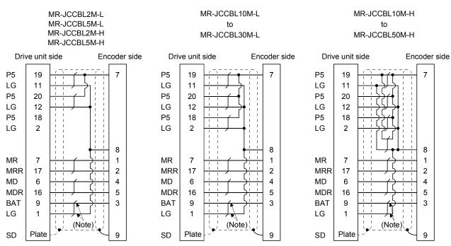
Note. Always make connection for use in an absolute position detection system. This wiring is not needed for use in an incremental system.
