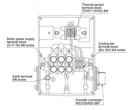
Terminal block signal arrangement
