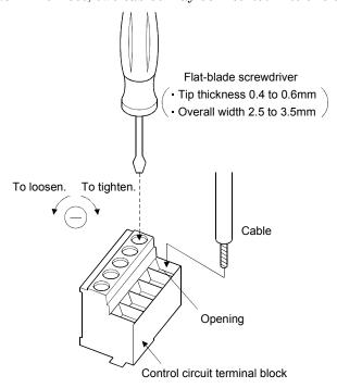
Use of a flat-blade torque screwdriver is recommended to manage the screw tightening torque. The following table indicates the recommended products of the torque screwdriver for tightening torque management and the flat-blade bit for torque screwdriver. When managing torque with a Phillips bit, please consult us.
