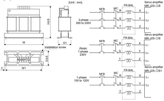
Note. For the 1-phase 230V power supply, Connect the power supply to L<sub>1</sub>, L<sub>2</sub> and leave L<sub>3</sub> open.
