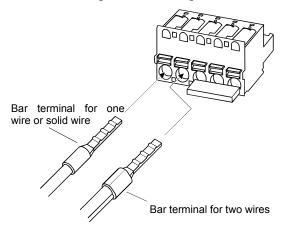
When two cables are inserted into one opening, a bar terminal for 2 cables is required.
