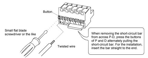
(b) When the twisted wires are put together using a bar terminal Insert a bar terminal with the odd-shaped side of the pressured terminal on the button side.
