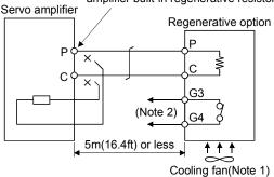
Note 1. When using the MR-RB50 • MR-RB51, forcibly cool it with a cooling fan (92 × 92, minimum air flow: 1.0m³).
