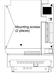
2) Remove the front cover mounting screws (2 places).
