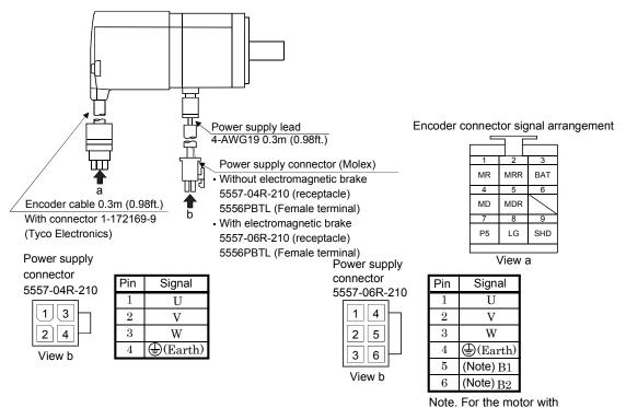
electromagnetic brake, supply electromagnetic brake power (24VDC). There is no polarity.
