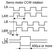
Time cycle (T) is determined by the settings of parameter No.33 and 38.
