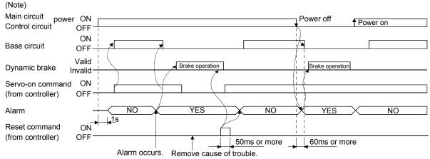
Note. Switch off the main circuit power as soon as an alarm occurs.
