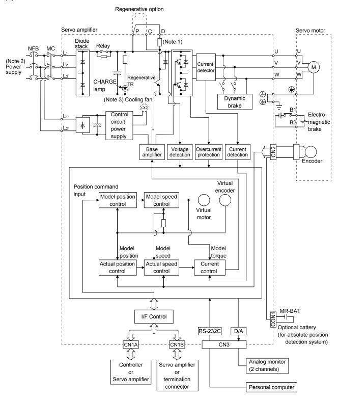
Note 1. The built-in regenerative resistor is not provided for the MR-J2S-10B (1).
