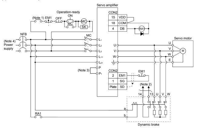
Note 1. Configure up the circuit to switch power off in the external sequence at servo alarm occurrence.
