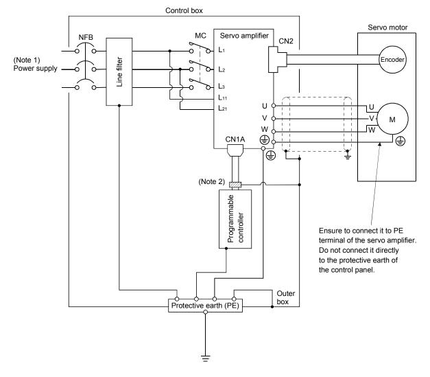
Note 1. For 1-phase 230V, connect the power supply to  $L_1 \cdot L_2$  and leave  $L_3$  open. There is no  $L_3$  for 1-phase 100 to 120V power supply. Refer to section 1.3 for the power supply specification.
