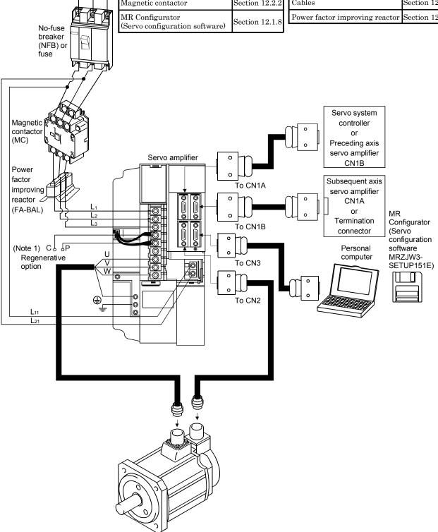
Note 1. When using the regenerative option, remove the lead wires of the built-in regenerative resistor.
