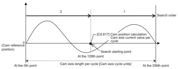
• Searches until between the 255th point and the 256th point (last point) in order of the cam data between the 128th point and the 129th point and between the 130th point and the 131th point.
