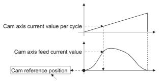
Restored by the equation of "Feed current value - Cam axis current value per cycle"
