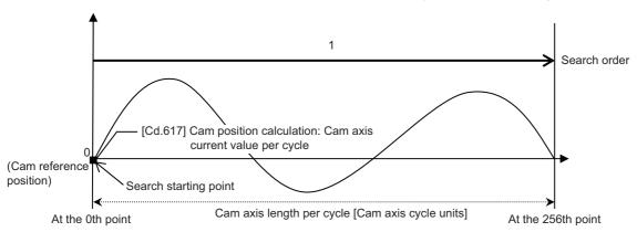
• Searches until between the 255th point and the 256th point (last point) in order of the cam data between the 0th point and the 1st point and between the 1st point and the 2nd point.
