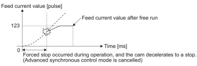
• Restore operation at restart of advanced synchronous control
