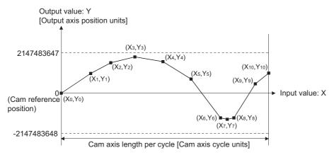
When an input value that is 0 or the cam axis length per cycle does not exist in the coordinate data, the coordinate is calculated from the line segment between the nearest two coordinates.
