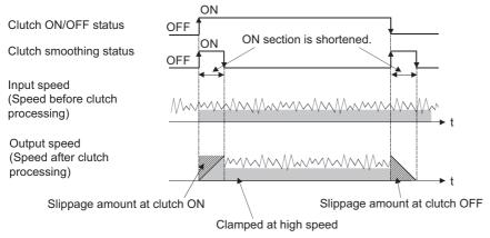
["5: Slippage method (Linear: Input value follow up)" is set.] The clutch smoothing status ON section is fixed.
