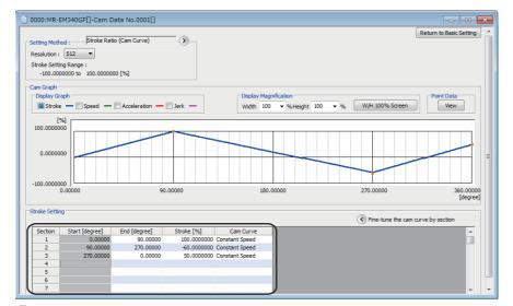
**5.** Select the Navigation window ⇒ "Synchronous Control Parameter" ⇒ "Synchronous Parameter" ⇒ "Axis #1 Synchronous Parameter", then set the synchronous parameter of the axis 1.
