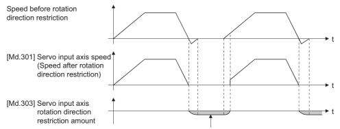
The input movement amount is accumulated as a rotation direction restricted amount, and will be reflected when the input movement amount in the enabled direction.
