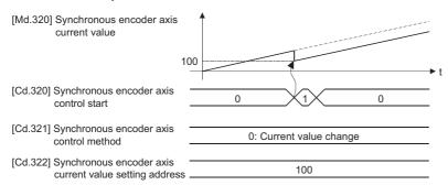
If set to "201", the synchronous encoder axis control starts based on the link device input assigned to the synchronous encoder axis start request by the link device external signal assignment function.
