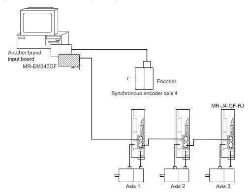
Set "201: Synchronous encoder via buffer memory" in "[Pr.320] Synchronous encoder axis type" of synchronous encoder axis 4
