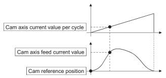
Select from 3 objects as follows in "[Pr.462] Cam axis position restoration object" which position is to be restored.
