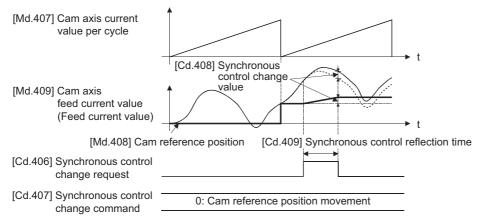
When "[Cd.406] Synchronous control change request" is reset to "0" while executing the cam reference position movement instruction, operation is stopped midway. If the cam reference position movement instruction is executed again, the remainder movement amount is not reflected, and the operation starts with "[Cd.408] Synchronous control change value" to be used again.
