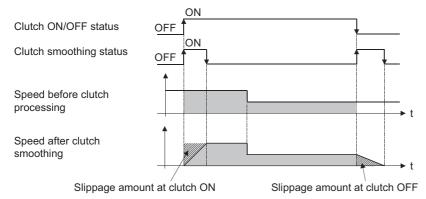
· When the input speed to the clutch is changed continuously and slightly
