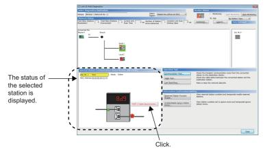
**5.** Various tests and operations can be performed by clicking the "Operation Test", "Information Confirmation/Setting", or "Selected Station Operation" on the bottom left of the window. ( Page 53 Link Start/Stop to Page 57 Enable/Disable Ignore Station Errors)
