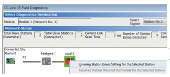
In "Network Status" of the "CC-Link IE Field Diagnostics" window, right-click the icon of the station to be set as a temporary error invalid station, and click "Ignoring Station Errors Setting for the Selected Station".
