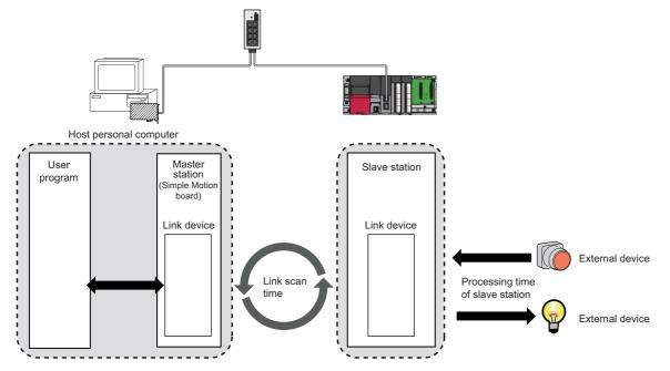
Slave station processing time: DManual for the slave station used
